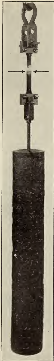
FIGURE 15.— Prolonged loading test on pretinned \frac{1}{2} -inch flat-lock seam Seam is indicated by the arrows.
