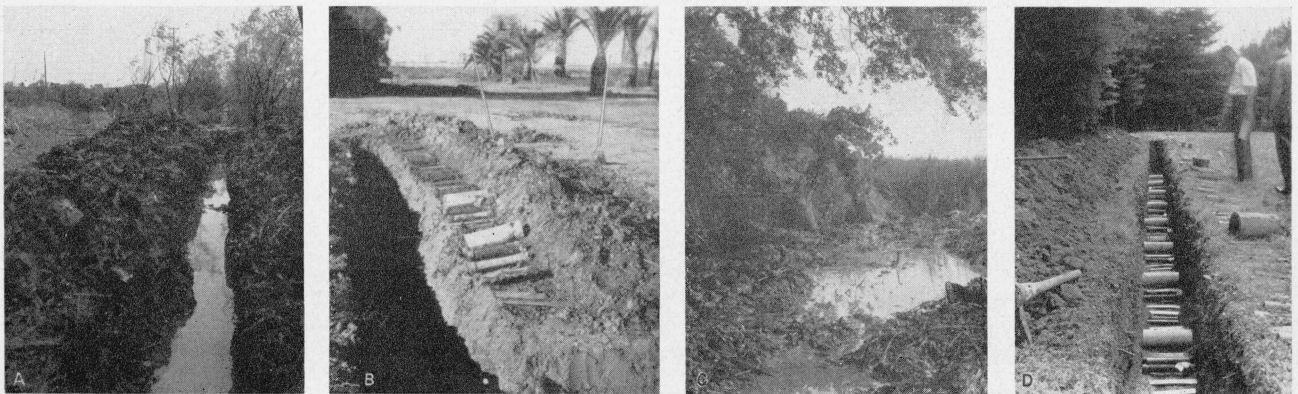
FIGURE 1. Test sites illustrating the environmental conditions to which specimens of asbestos-cement pipe were exposed.
