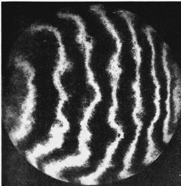
FIGURE 8. Topographic map of one optical surface, relative to a standard, produced by photographing a given fringe (order of interference) successively, as it was moved across the plate, by controlled evacuation of air wedge between the plates.
