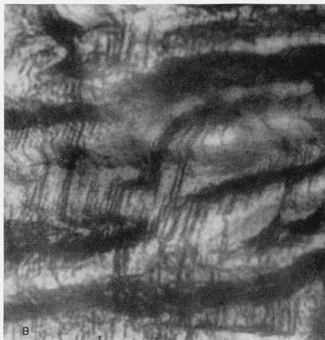
FIGURE 11. Intragranular structure of a specimen tested in tension at 80° F with a strain rate of 60,000 percent per 1,000 hr; longitudinal sections, 0.1 in. from complete fracture, etched in 10 parts nitric acid (concentrated), 10 parts hydrochloric acid (concentrated), 3 parts hydrofluoric acid (47%), and 77 parts water.
