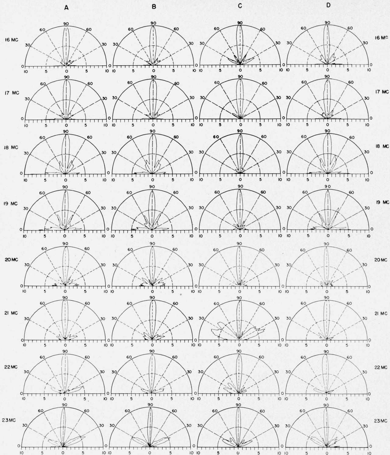
FIGURE 4—Continued. Normalized radiation patterns in space for a multiple-wire delta antenna supported by an insulated mast and for a multiple-wire delta antenna supported by a metal mast with and without guy wires.
