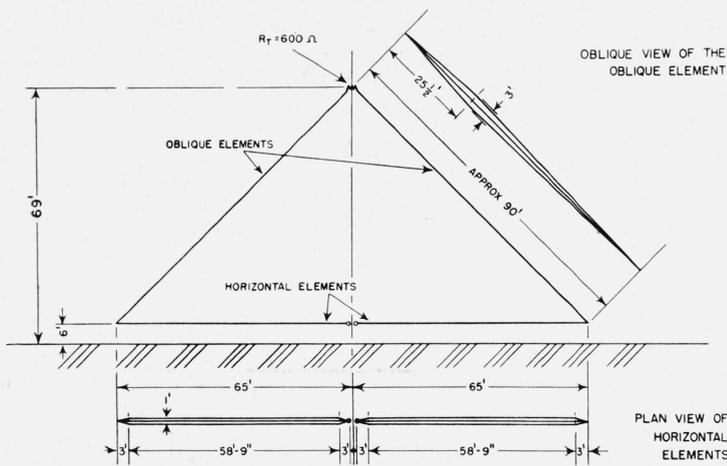
FIGURE 1. Simplified diagram of the 600-ohm multiple-wire delta antenna.
