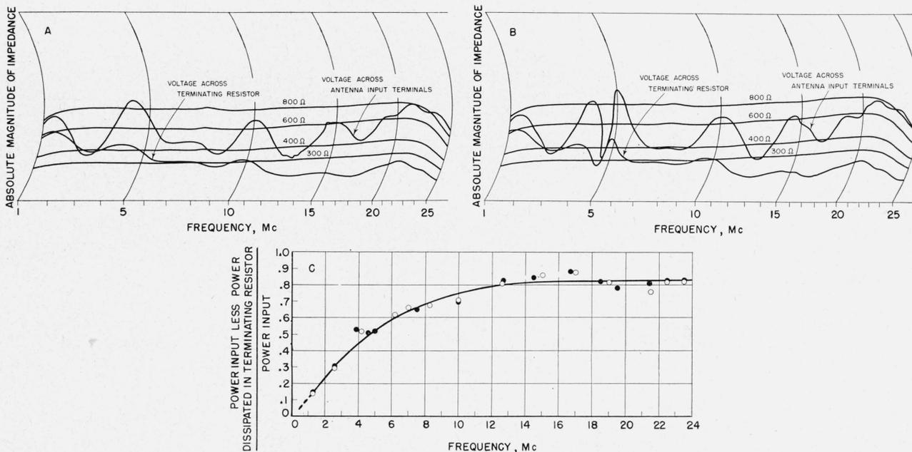
FIGURE 7. Measurements of the quasi-radiation efficiency of a multiple-wire delta antenna with and without guy wires.
