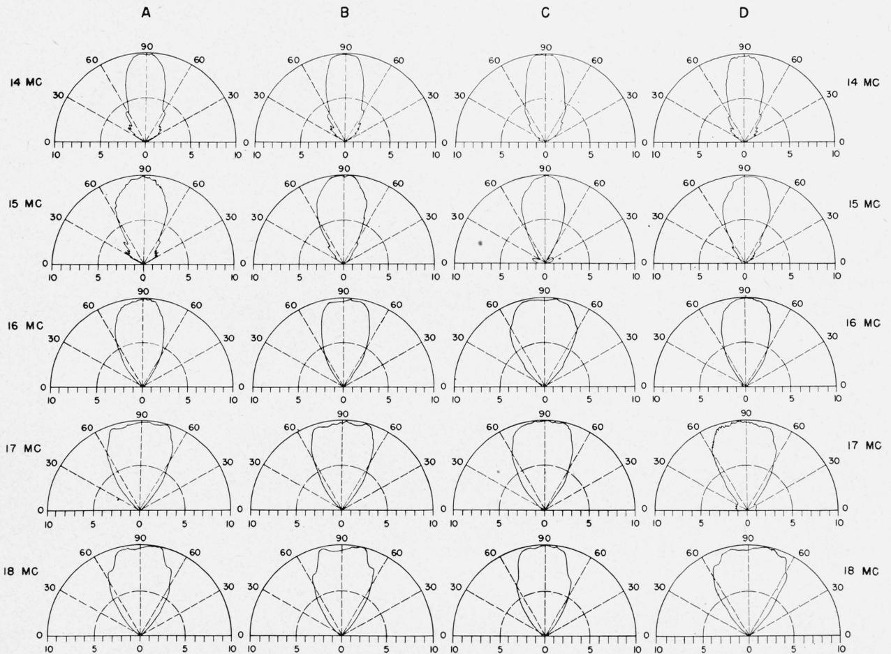
FIGURE 5. Normalized radiation patterns in space for a multiple-wire delta antenna supported by an insulated mast and for a multiple-wire delta antenna supported by a metal mast with and without guy wires.
