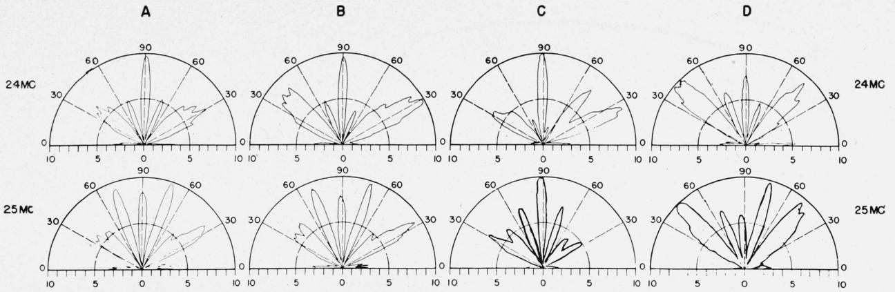
FIGURE 4—Continued. Normalized radiation patterns in space for a multiple-wire delta antenna supported by an insulated mast and for a multiple-wire delta antenna supported by a metal mast with and without guy wires.
