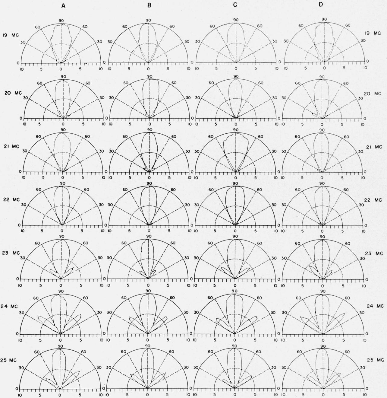
FIGURE 5—Continued. Normalized radiation patterns in space for a multiple-wire delta antenna supported by an insulated mast and for a multiple-wire delta antenna supported by a metal mast with and without guy wires.
