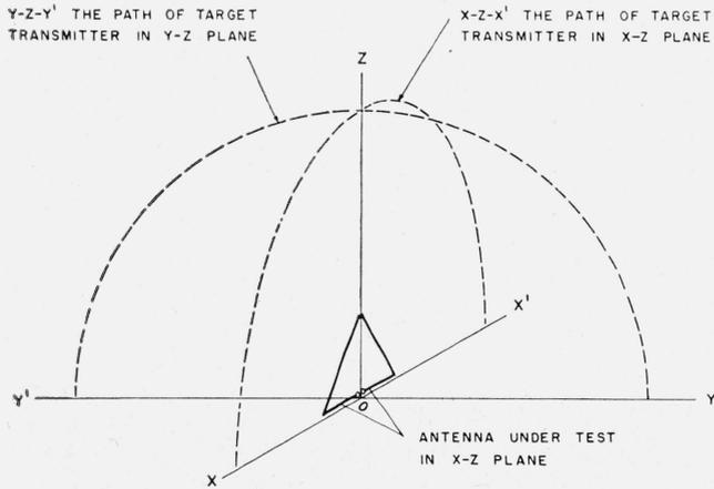
FIGURE 3. Diagram of the model range showing the paths of the target transmitter with reference to the antenna under test.
