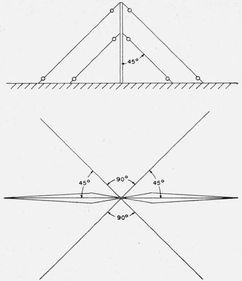
FIGURE 2. Arrangement of guy wires used with multiple-wire delta antenna.
