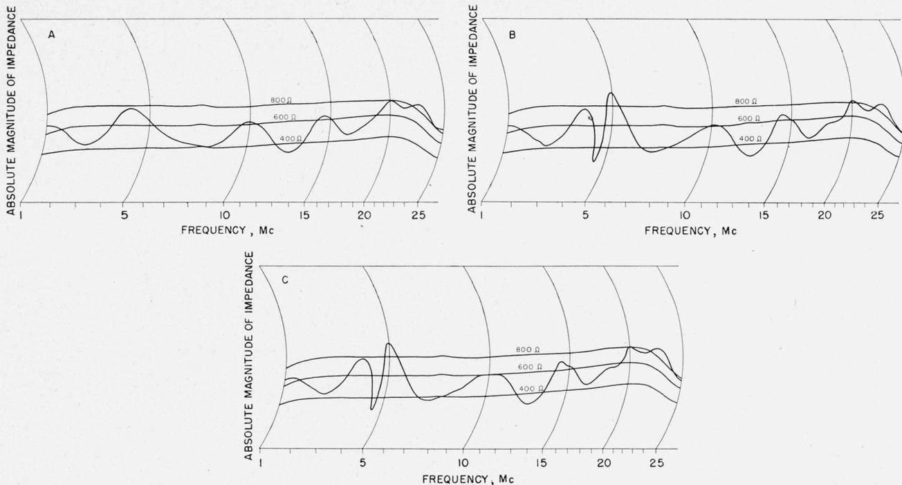
FIGURE 6. Impedance of 600-ohm multiple-wire delta antenna with and without guy wires.
