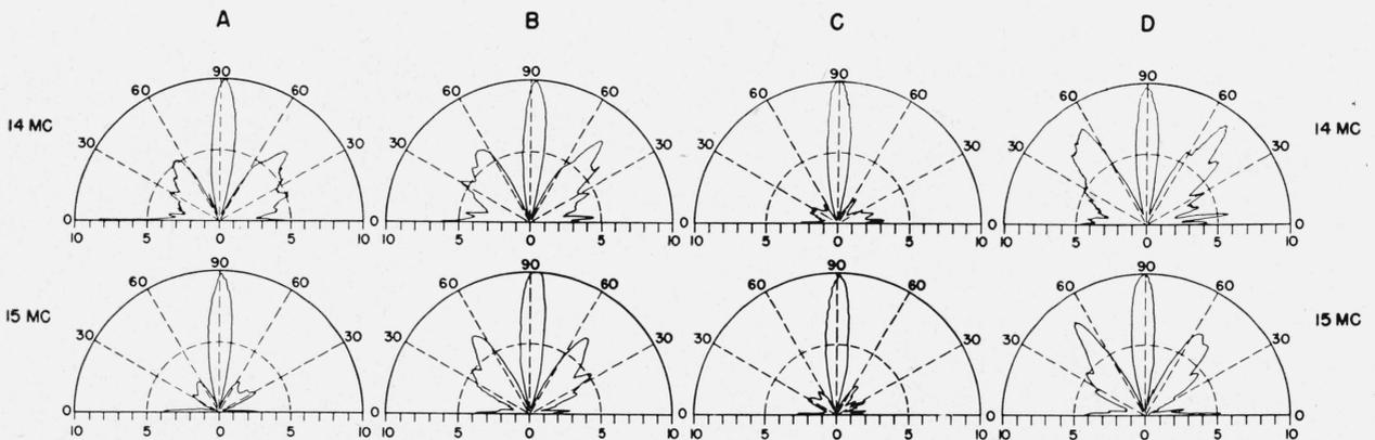
FIGURE 4. Normalized radiation patterns in space for a multiple-wire delta antenna supported by a metal mast with and without guy wires.
