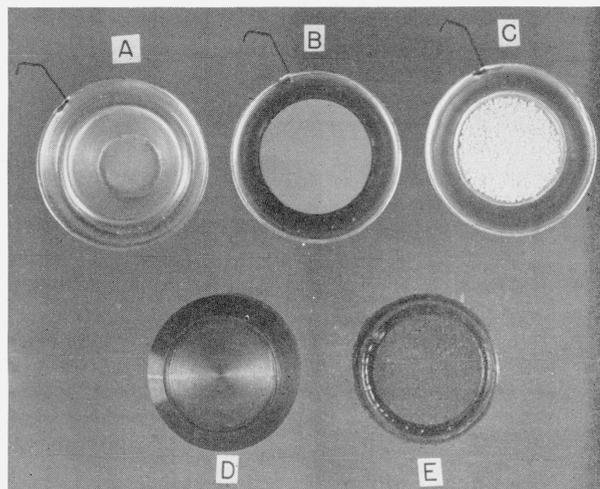
FIGURE 1. A, Empty aluminum cell used in the water vapor permeability studies; B, assembled cell and leather specimen ready for measurements; C, assembled cell with transparent cellulose film showing desiccant; D, template used in assembling the cell; E, side of leather specimen next to desiccant after determination of water vapor permeability was made.
