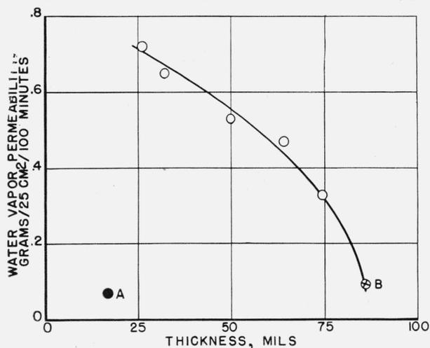
FIGURE 10. Effect of thickness on water vapor permeability when increments of the grain side are split off. A, Grain split; B, full thickness; rest, flesh splits; ○, grain split off; ●, flesh split off; grain removed first.
