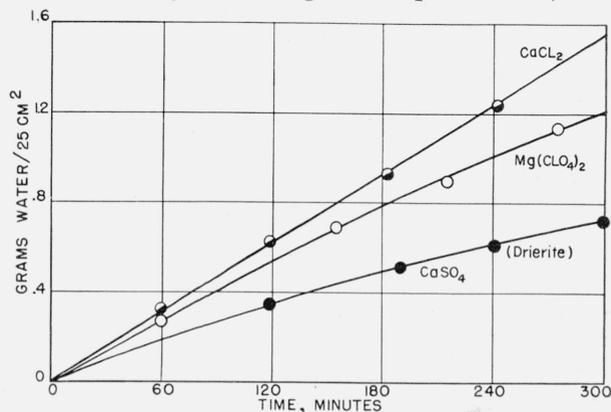
FIGURE 2. Rate of moisture pickup by various desiccants used in the cells.
