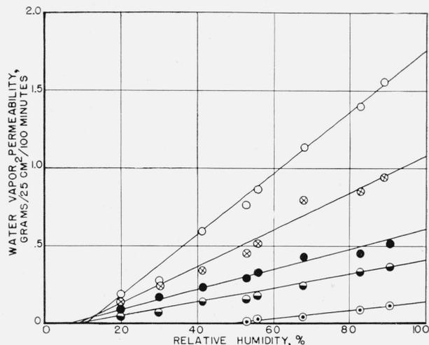
FIGURE 11. Influence of relative humidity on water vapor permeability.
