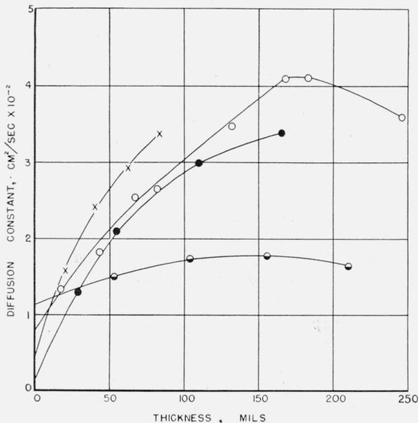
FIGURE 4. Change of the diffusion constant of glass cloth, leather, cotton duck, and nylon with thickness. X, Glass cloth; O, leather; ●, cotton duck; ◐, nylon.
