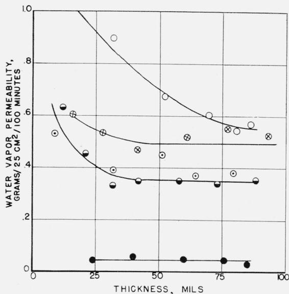
FIGURE 9. Effect of grease content and thickness on the water vapor permeability of upper leather.
