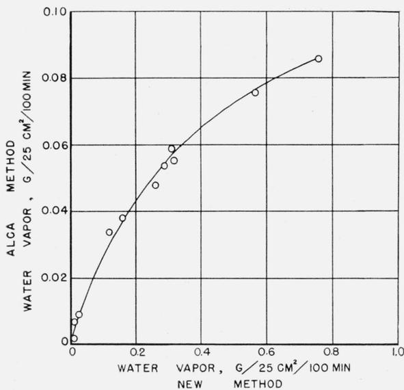
FIGURE 3. Correlation of ALCA method with the new method for determining water vapor permeability.
