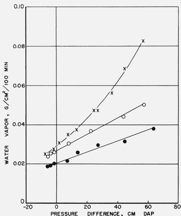
FIGURE 17. Influence of flexing on the water vapor permeability of upper leather containing a high percentage of grease.
