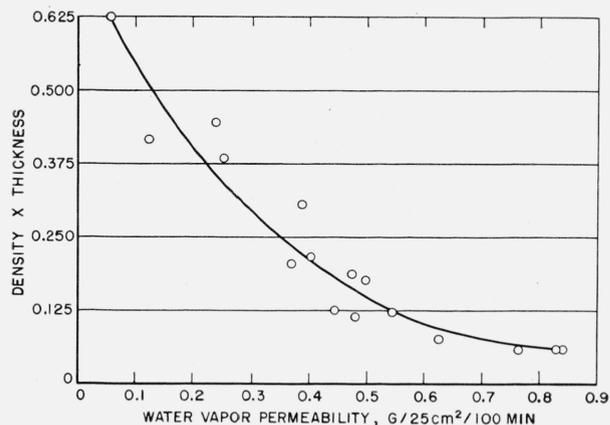
FIGURE 12. Correlation of the water vapor permeability of leather with the product of the density and the thickness in centimeters.
