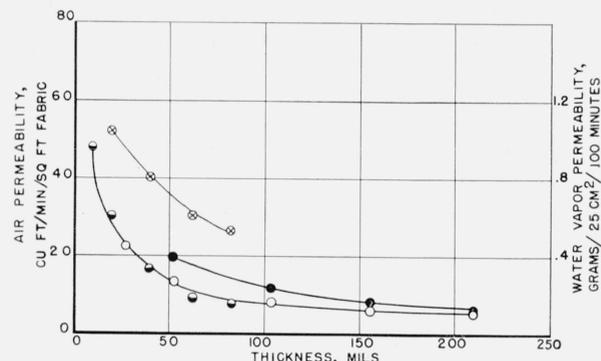
FIGURE 7. Comparison of the air permeability and the water vapor permeability of glass and nylon fabrics as a function of thickness.
