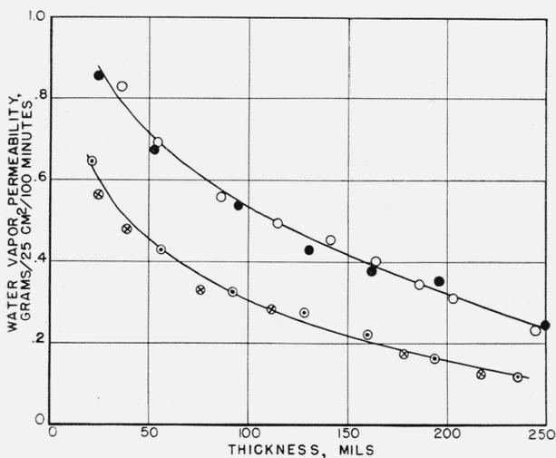
FIGURE 8. Effect of thickness on the water vapor permeability of leather.
