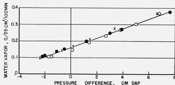
FIGURE 16. Influence of flexing on the water vapor permeability of degreased upper leather.
