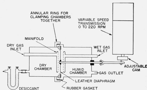
FIGURE 15. Sketch of the equipment used to determine water vapor permeability under dynamic conditions.
