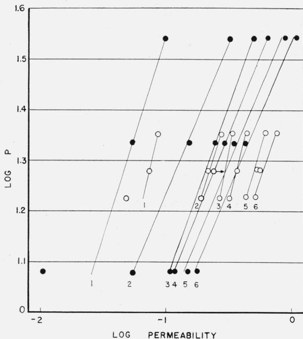
FIGURE 13. Influence of temperature on water vapor permeability.
