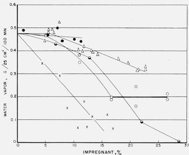
FIGURE 14. Effect of various leather impregnants on the water vapor permeability.
