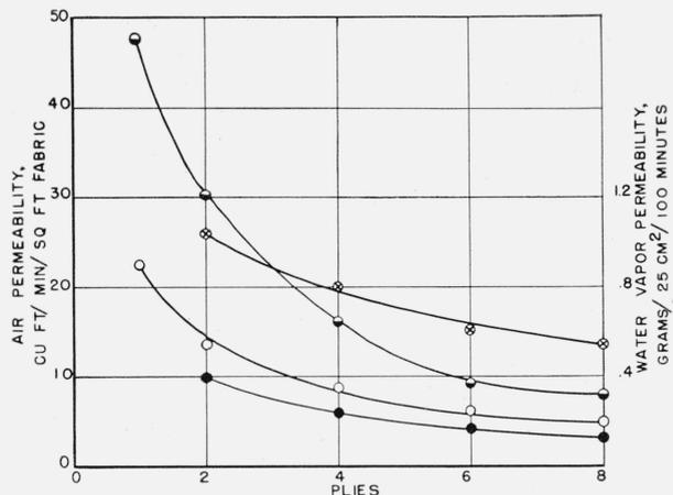
FIGURE 6. Comparison of the air permeability and the water vapor permeability of glass and nylon fabrics, as a function of number of plies.
