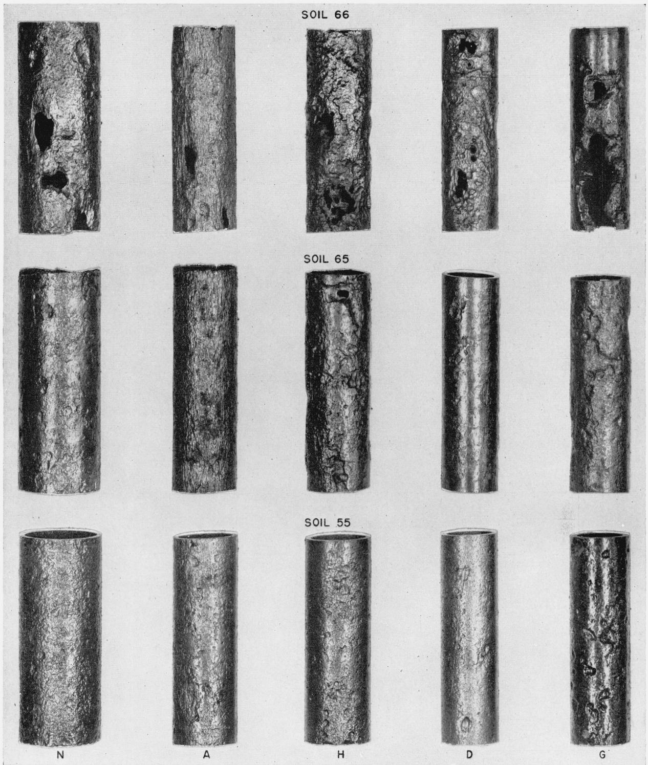
FIGURE 2. Corrosion of steel, cast iron, and low-alloy iron and steel in soils differing in corrosiveness—exposure 14 yr. N, Carbon steel; A, hand-puddled wrought iron; H, Cu-Mo open-hearth iron; D, 2-percent Ni, 1-percent Cu steel; G, cast iron.
