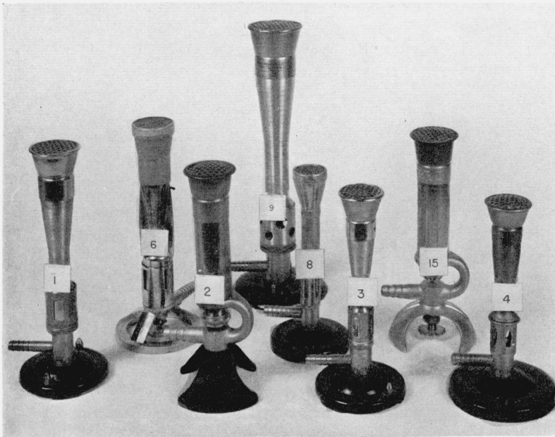
FIGURE 1. Laboratory burners tested. Meker type.
