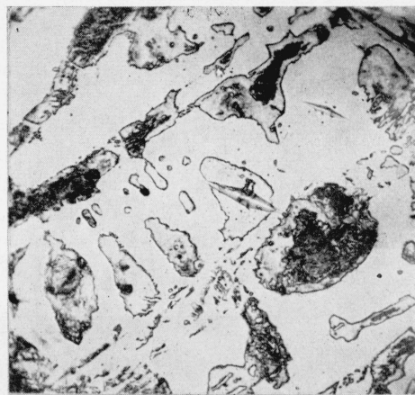
FIGURE 13. Micrograph showing Knoop hardness indentations on different structural components of transverse test bar cast from stock iron G-137.
