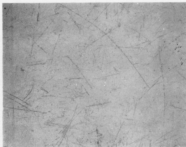
FIGURE 13. Print from a replica of a china plate after 10 years of service.
