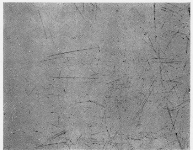
FIGURE 11. Print from a replica of an acid-resisting cast-iron sink after approximately 1 year of service.
