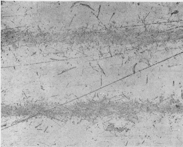
FIGURE 8. Print from a replica of the corrugated drain-board of an enameled cast-iron sink.
