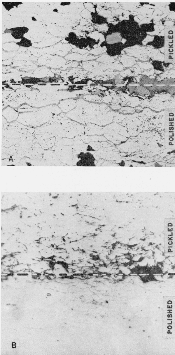
FIGURE 1. Effect of method of scale removal on susceptibility to intergranular attack.
