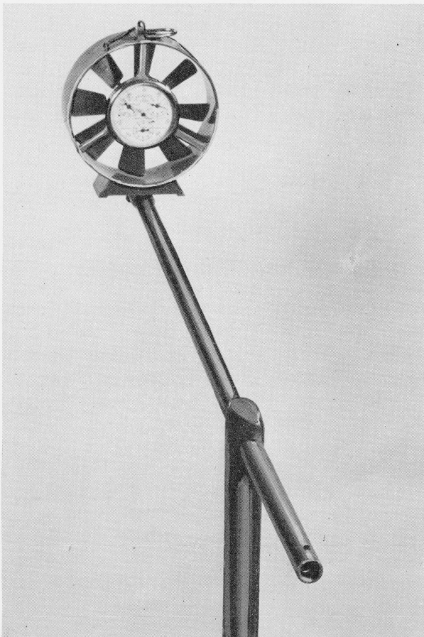
FIGURE 2. Anemometer supported on rod.
