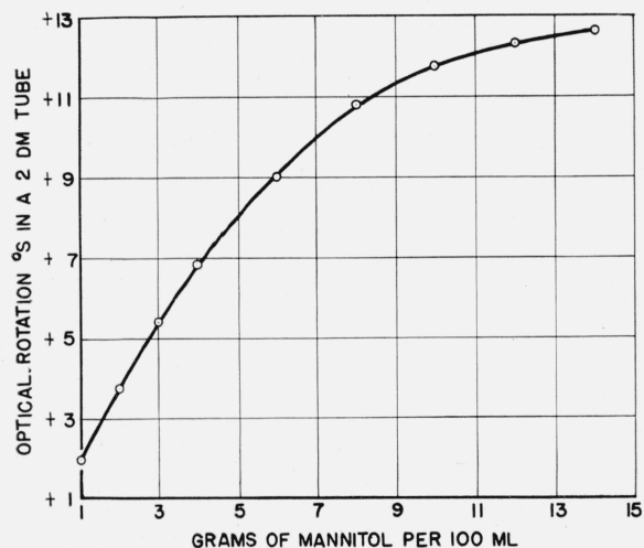
FIGURE 12. Optical rotation of mannitol in the presence of 10 g of Na 2 B 4 O 7 ·10H 2 O per 100 ml of solution.
