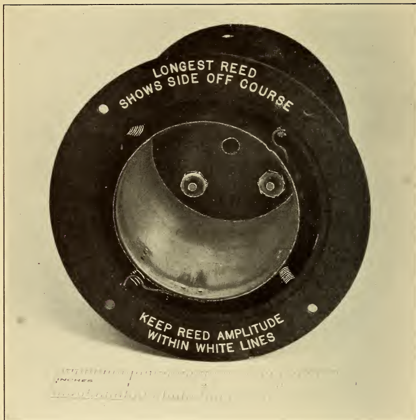
FIGURE 7.—Cylindrical type of shock-proof mounting for 12-course tuned reed indicator shown in Figure 6
