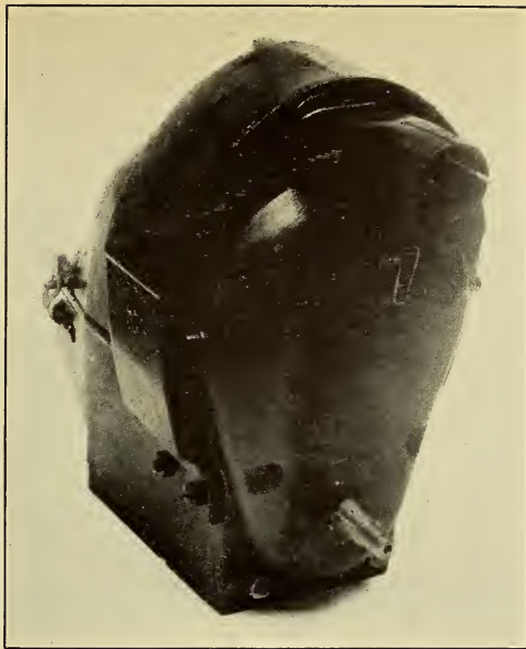
FIGURE 12.— Completely shielded magneto used in installation of Figure 8 with side entrance for the ignition distributing leads
