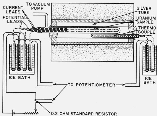
FIGURE 1.—Diagram of apparatus
