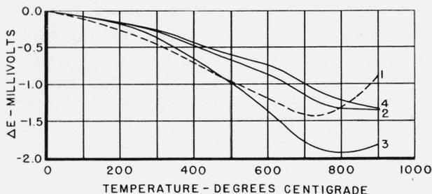
FIGURE 4.—Differences in thermal electromotive force of uranium samples.
