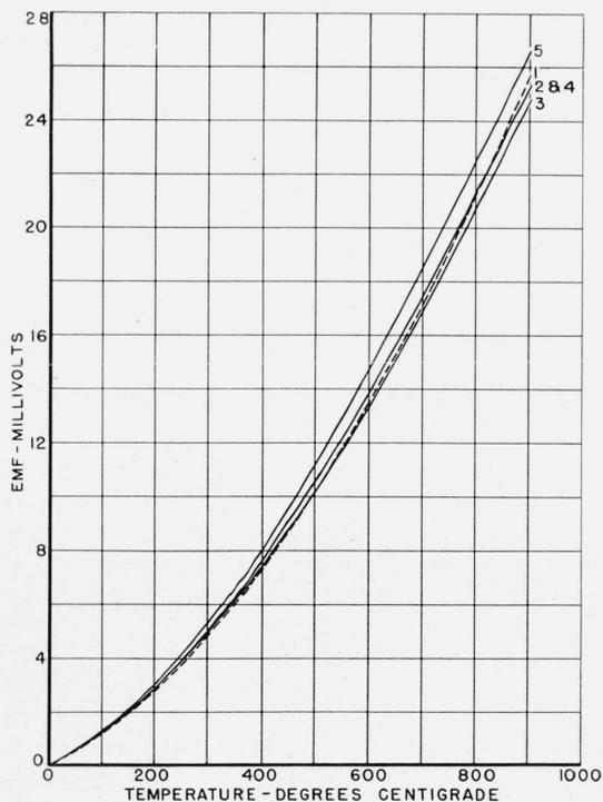
FIGURE 3.—Thermal electromotive force of uranium versus platinum.
