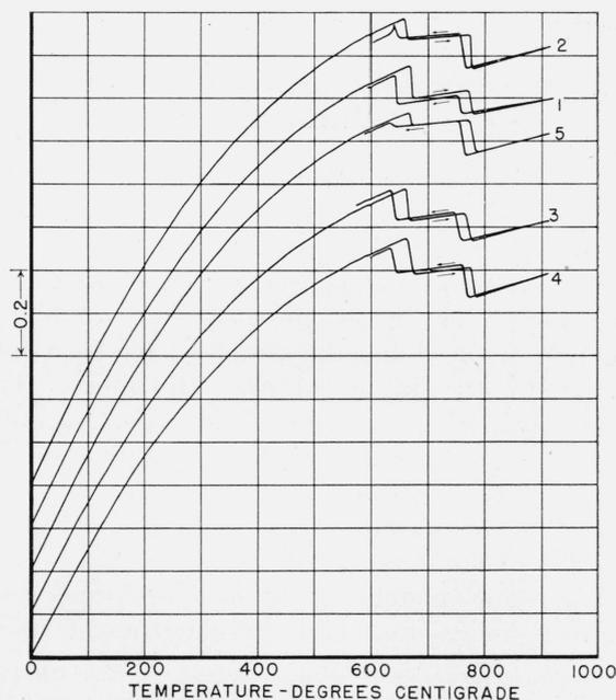
FIGURE 2.—Resistance-temperature relation for uranium.
