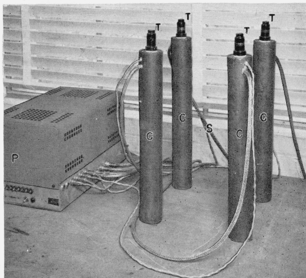
FIGURE 1.—View of counters and scaler assembled for use.
