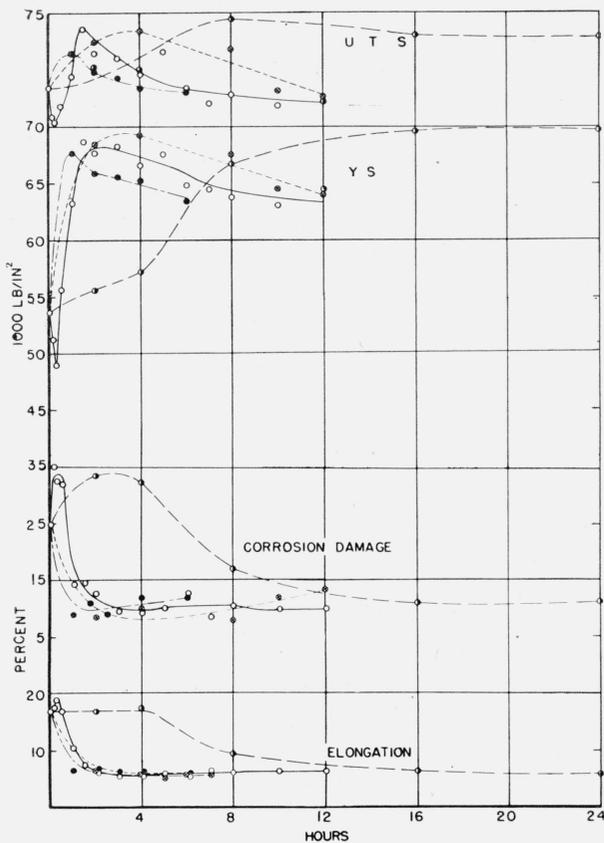
FIGURE 19.—Relationship between aging time and tensile properties of parallel A specimens.
