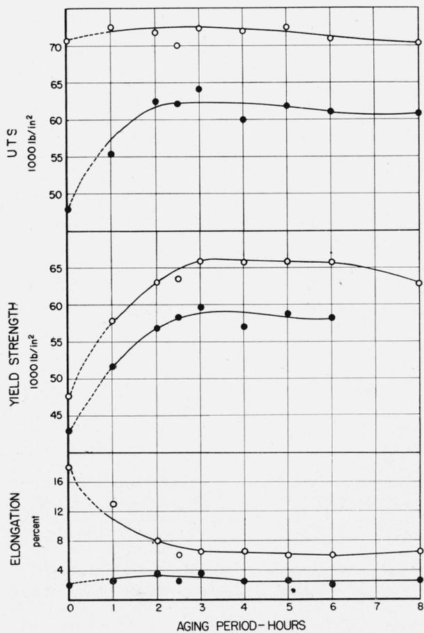
FIGURE 7.—Tensile properties of transverse specimens of A material, aged at 385° F, before and after exposure for 24 hr in the NaCl+H<sub>2</sub>O<sub>2</sub> solution.
