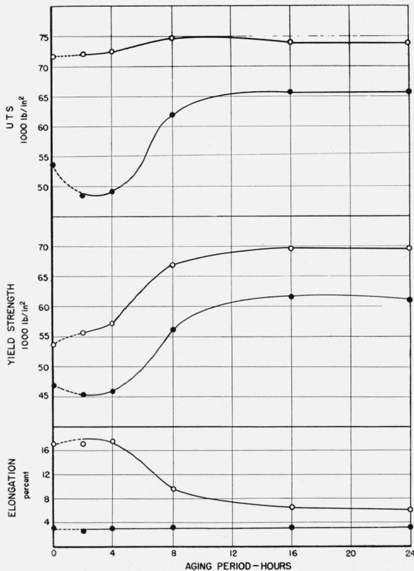
FIGURE 15.—Tensile properties of parallel A specimens, aged at 350° F, before and after exposure for 24 hr in the NaCl+H<sub>2</sub>O<sub>2</sub> solution.
