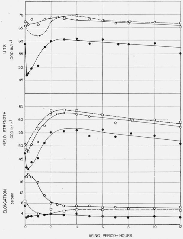
FIGURE 6.—Tensile properties of parallel specimens of B material, aged at 385° F, before and after exposure (anodized) to a marine atmosphere for 6 weeks and in the NaCl+H<sub>2</sub>O<sub>2</sub> solution without surface protection for 24 hr.
