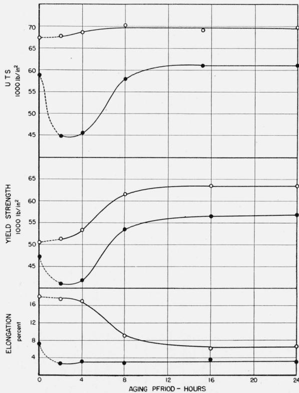
FIGURE 16.—Tensile properties of parallel B specimens, aged at 350° F, before and after exposure for 24 hr in the NaCl+H<sub>2</sub>O<sub>2</sub> solution.
