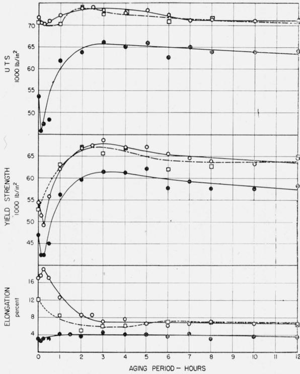
FIGURE 5.—Tensile properties of parallel specimens of A material, aged at 385° F, before and after exposure (anodized) to a marine atmosphere for 6 weeks and in the NaCl+H<sub>2</sub>O<sub>2</sub> solution without surface protection for 24 hr.
