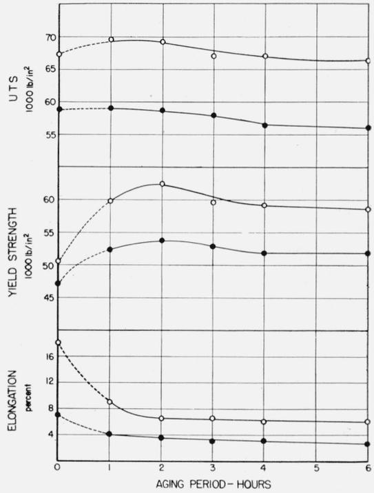
FIGURE 18.—Tensile properties of parallel B specimens, aged at 400° F, before and after exposure for 24 hr in the NaCl+H<sub>2</sub>O<sub>2</sub> solution.
