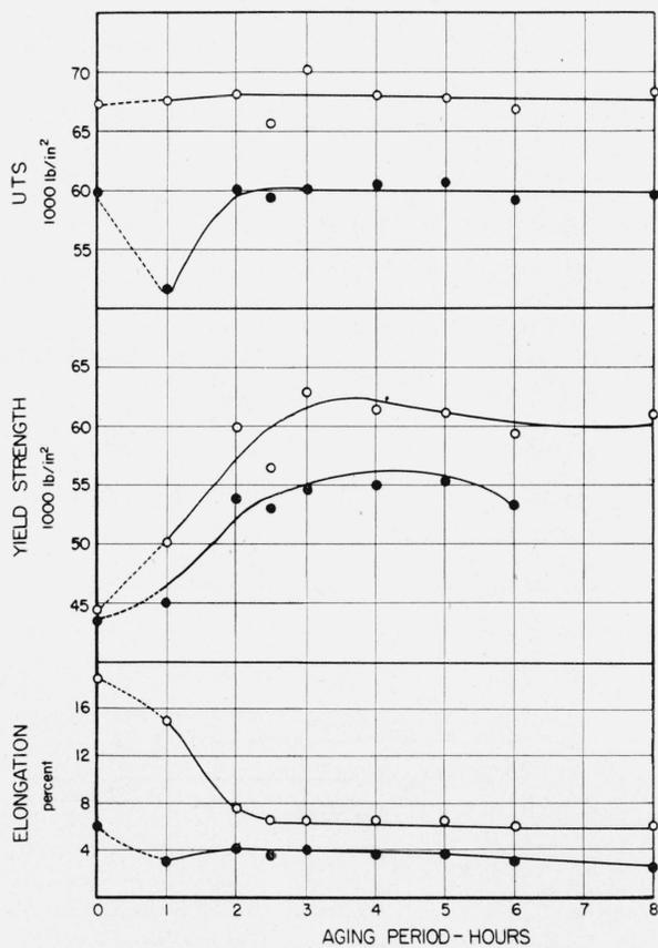
FIGURE 8.—Tensile properties of transverse specimens of B material, aged at 385° F, before and after exposure for 24 hr in the NaCl+H<sub>2</sub>O<sub>2</sub> solution.
