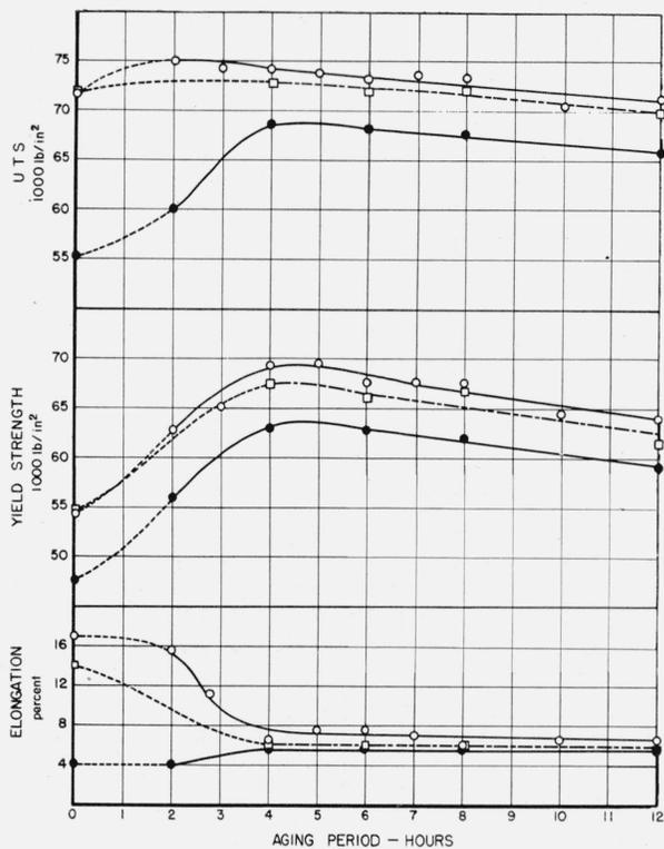
FIGURE 11.—Tensile properties of parallel A specimens, aged at 375° F, before and after exposure in a marine atmosphere for 6 weeks and in the NaCl+H<sub>2</sub>O<sub>2</sub> solution for 24 hr.
