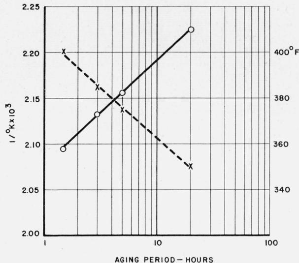
FIGURE 22.—Relationship between aging temperature and aging period necessary to produce maximum yield strengths.
