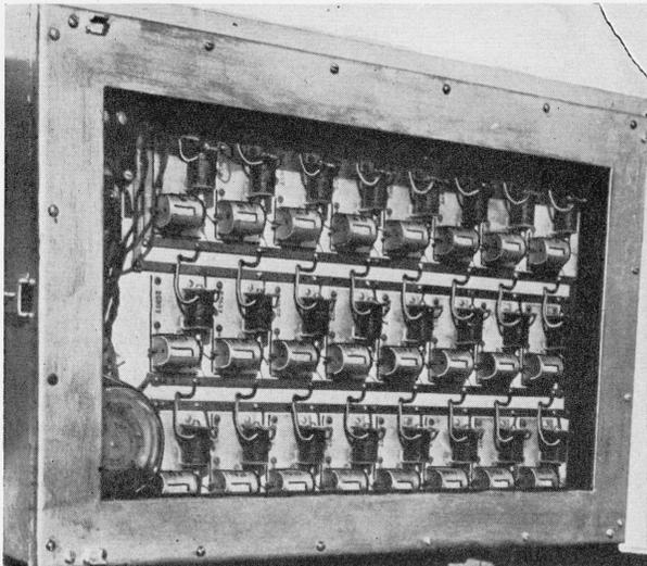
FIGURE 4.—Electric solenoid counters and time switch (lower left).
