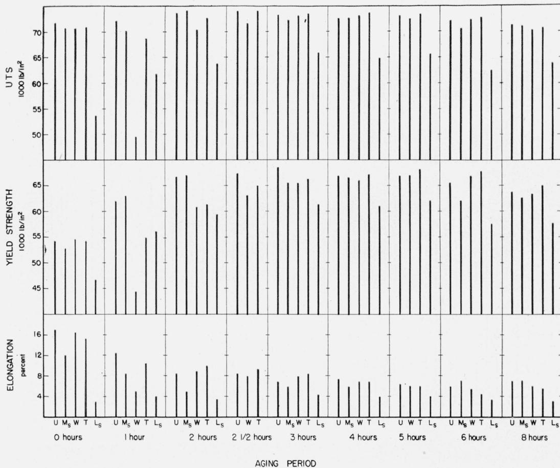
FIGURE 9.—Tensile properties of parallel specimens of A material aged at 385° F.
