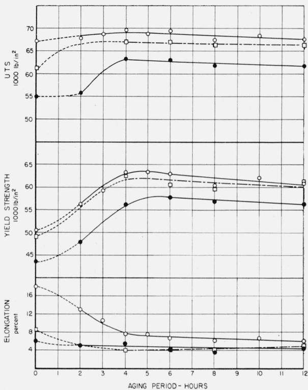
FIGURE 12.—Tensile properties of parallel B specimens, aged at 375° F, before and after exposure in a marine atmosphere for 6 weeks and in the NaCl+H<sub>2</sub>O<sub>2</sub> solution for 24 hr.
