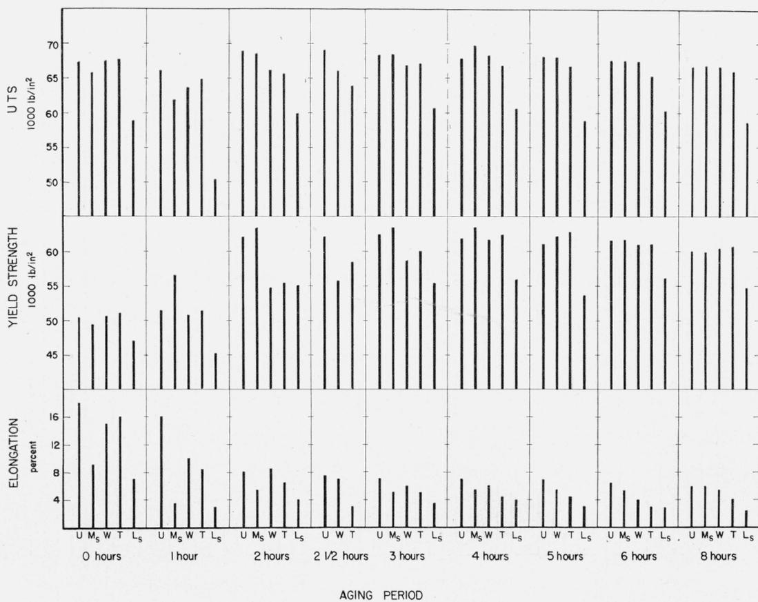
FIGURE 10.—Tensile properties of parallel specimens of B material aged at 385° F.
