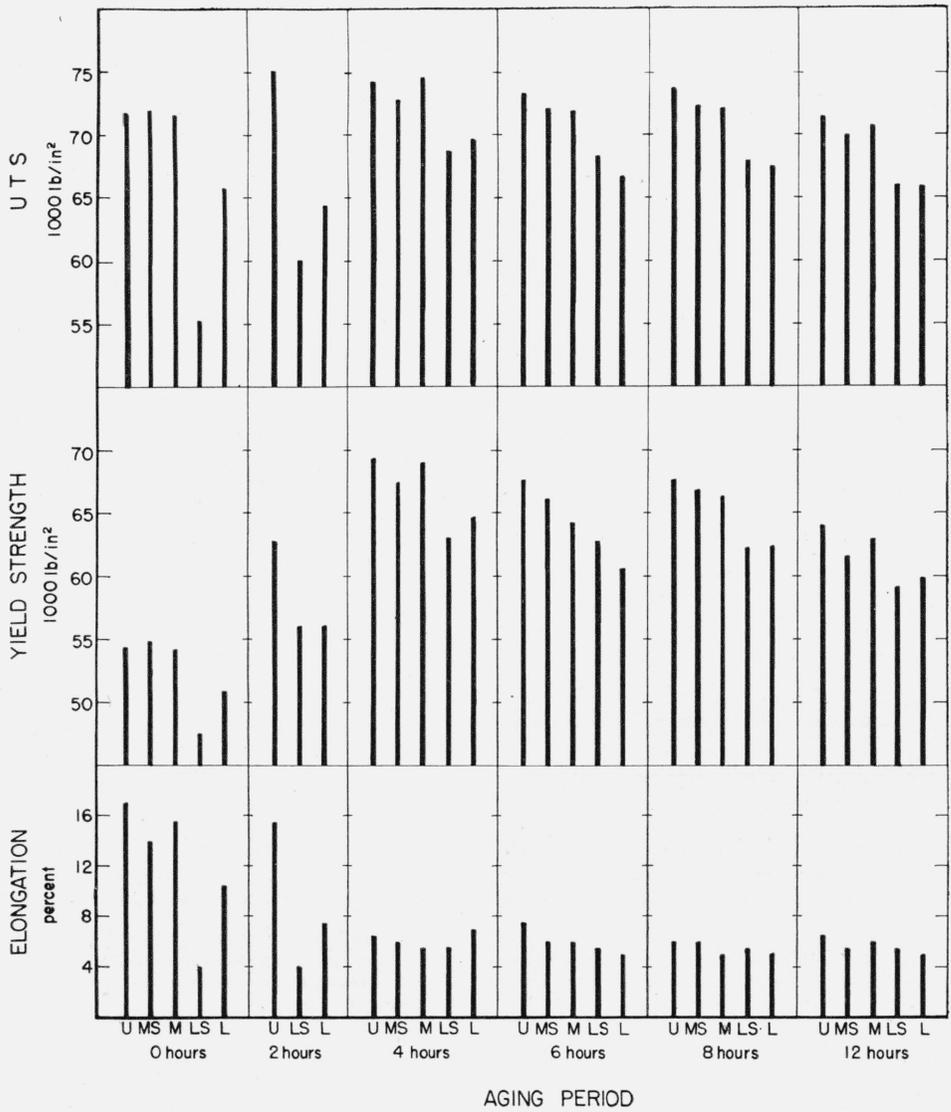
FIGURE 13.—Effect of stress and corrosion on tensile properties of parallel A specimens aged at 375° F.
