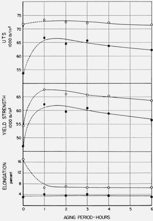
FIGURE 17.—Tensile properties of parallel A specimens, aged at 400° F, before and after exposure for 24 hr in the NaCl+H<sub>2</sub>O<sub>2</sub> solution.
