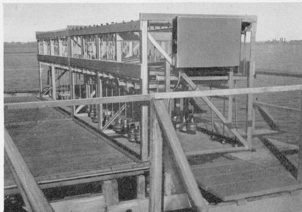
FIGURE 2.—Stress-corrosion racks, Naval Air Station, Hampton Roads, Va.
