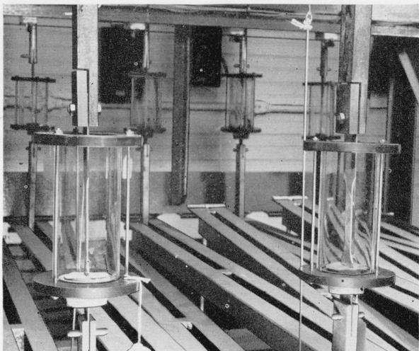
FIGURE 1.—Stress-corrosion rack with cells in place for tests in the  $\text{NaCl} + \text{H}_2\text{O}_2$  solution.
