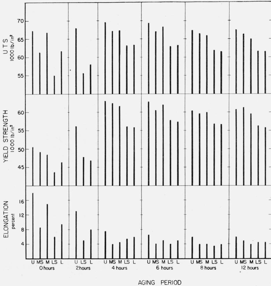
FIGURE 14.—Effect of stress and corrosion on tensile properties of parallel B specimens aged at 375° F.
