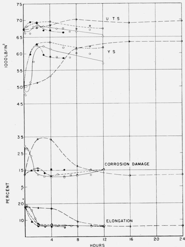
FIGURE 20.—Relationship between aging time and tensile properties of parallel B specimens.
