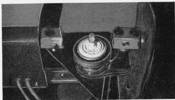
FIGURE 5.—Ceramic base and specimen holder.
