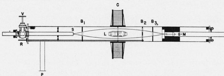
FIGURE 1.—Longitudinal section of thin magnetic-lens spectrometer.
