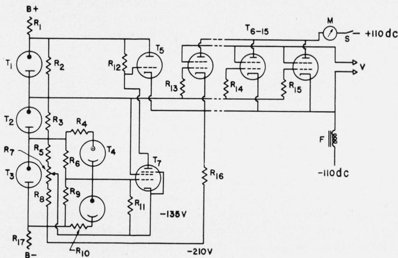
FIGURE 2.—Diagram of circuit for stabilizing current in the lens coils of the spectrometer.
