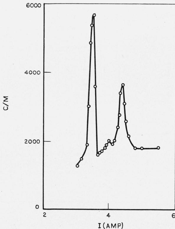
FIGURE 4.—Spectrum of conversion electrons from ThB+C deposit used for calibration.
