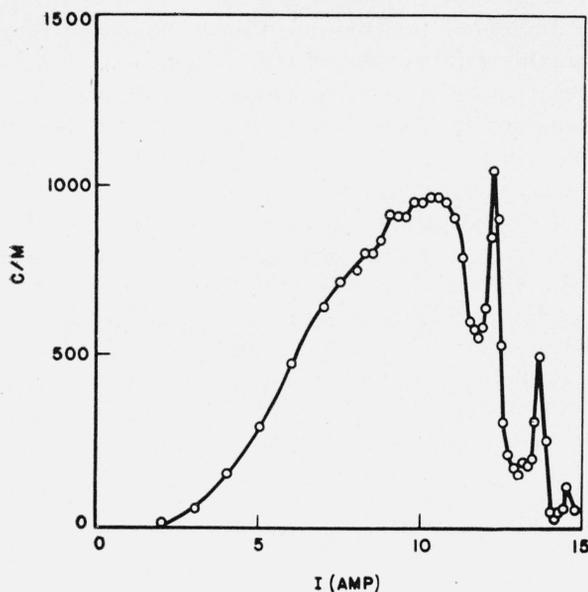
FIGURE 6.—Spectrum showing the conversion spectrum for  $\text{Co}^{60}$  gamma rays in uranium radiator, of thickness 23  $\text{mg}/\text{cm}^2$ .
