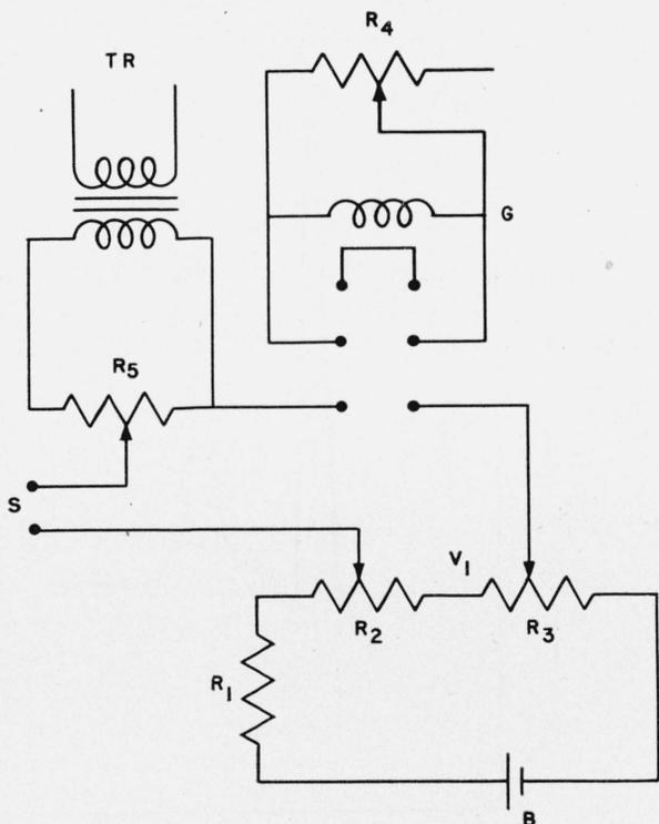
FIGURE 3.—Diagram of circuit for the photocell galvanometer.
