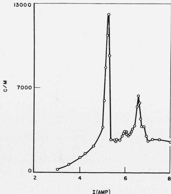
FIGURE 5.—Spectrum of conversion electrons from ThB+C deposit used for calibration.
