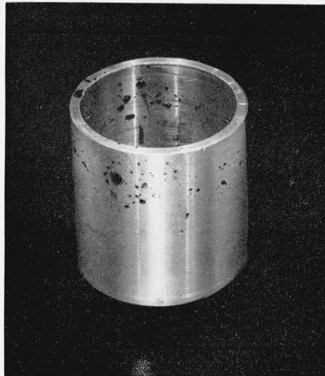
FIGURE 3.—Porous aluminum casting showing the exudation of resin that occurred during curing.
