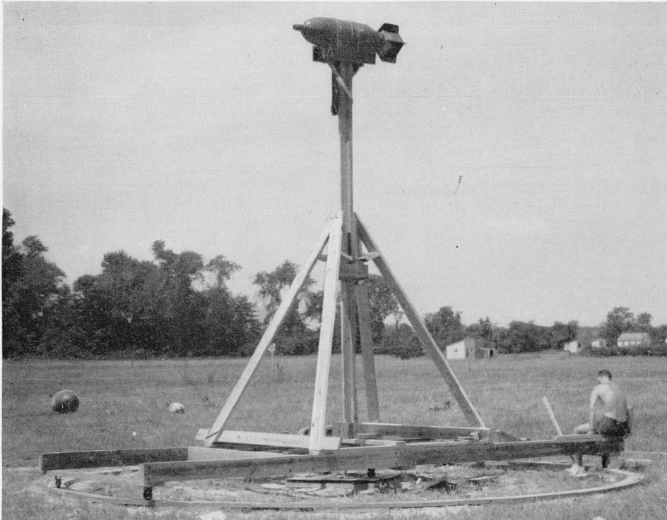
FIGURE 6.—Test structure for obtaining fuze directivity envelope.
