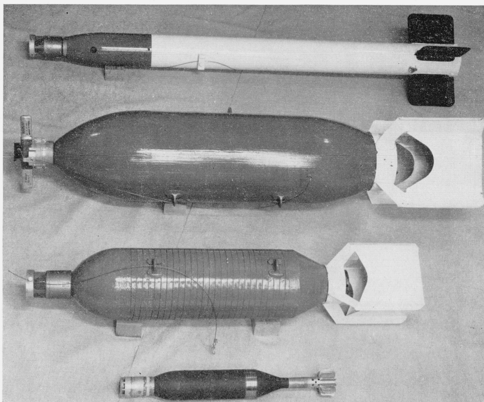
FIGURE 1.—Radio proximity fuzes mounted on high-velocity aircraft rocket, 500- and 265-lb bombs, and 81-mm trench mortar.
