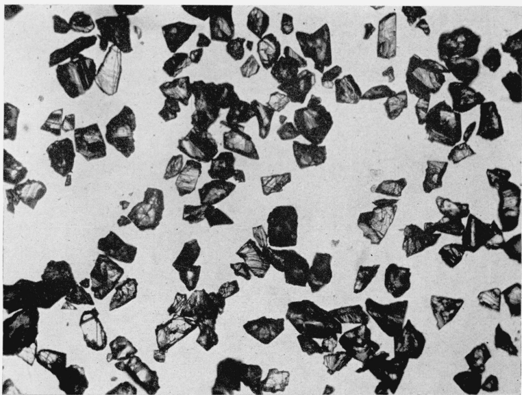
FIGURE 2.— Sieved fraction of diamond powder through No. 270 sieve and retained on No. 325.
