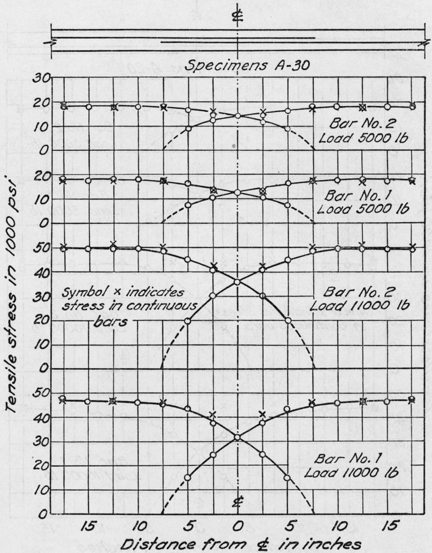
FIGURE 7.—Distribution of stress along lapped bars.
