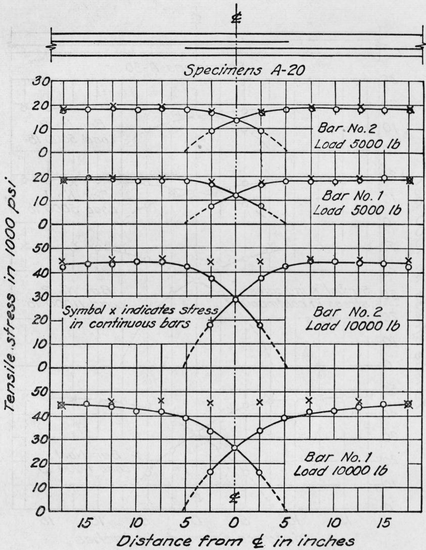
FIGURE 6.—Distribution of stress along lapped bars.
