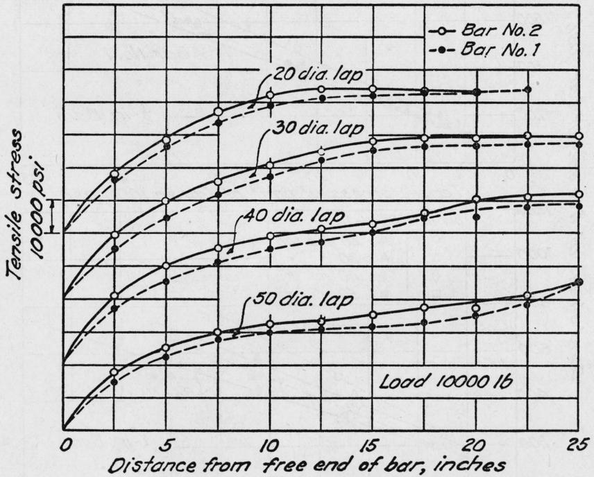
FIGURE 16.—Distribution of stress along lapped bars compared for No. 2 and No. 1  $\frac{1}{2}$ -in. bars.
