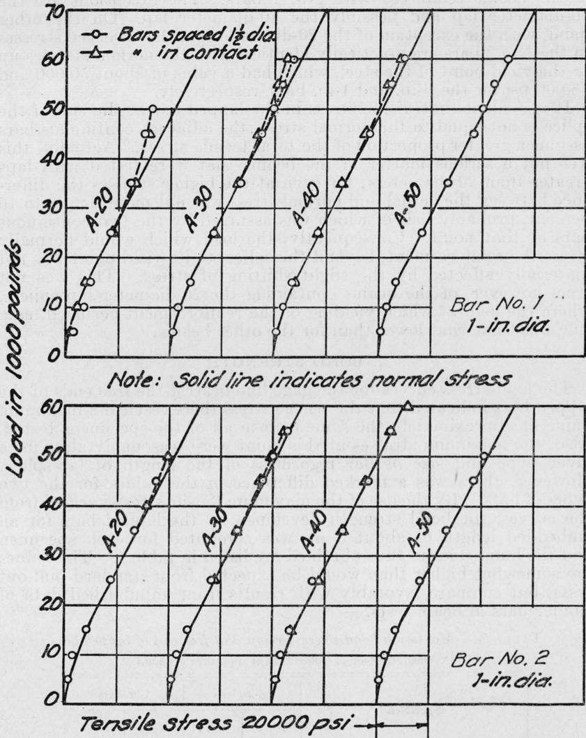
FIGURE 19.—Load-stress relation for lapped bars at limits of the splice.
