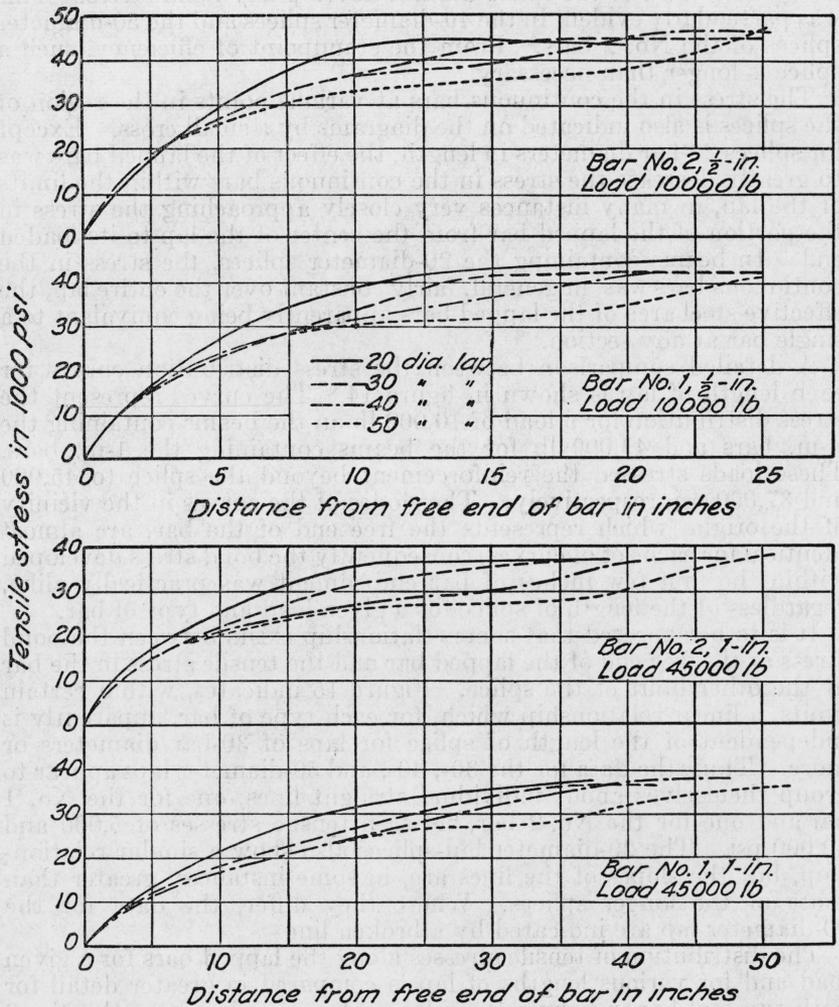
FIGURE 14.—Distribution of stress along lapped bars for various lengths of splice.
