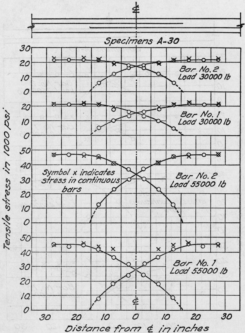
FIGURE 11.—Distribution of stress along lapped bars.
