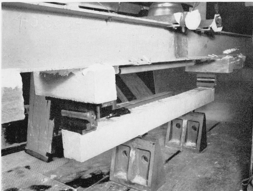
FIGURE 3.—Eight-foot beam of series A under load.
