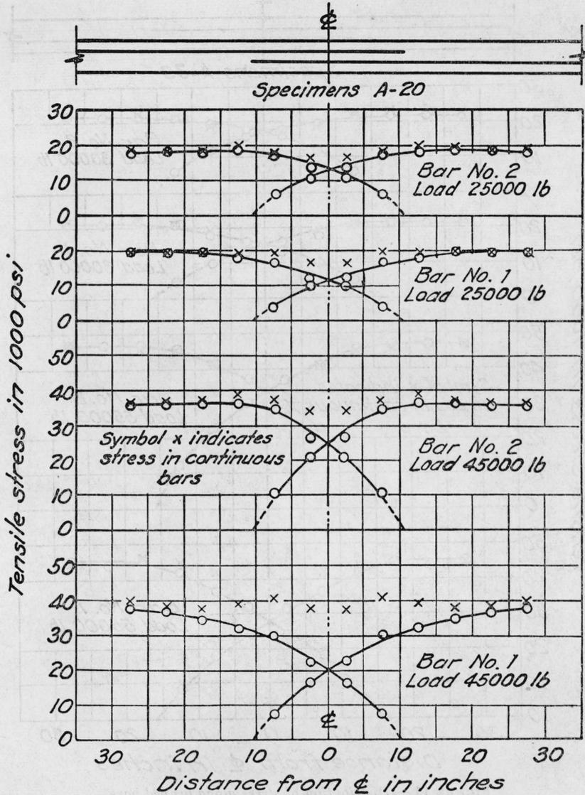
FIGURE 10.—Distribution of stress along lapped bars.
