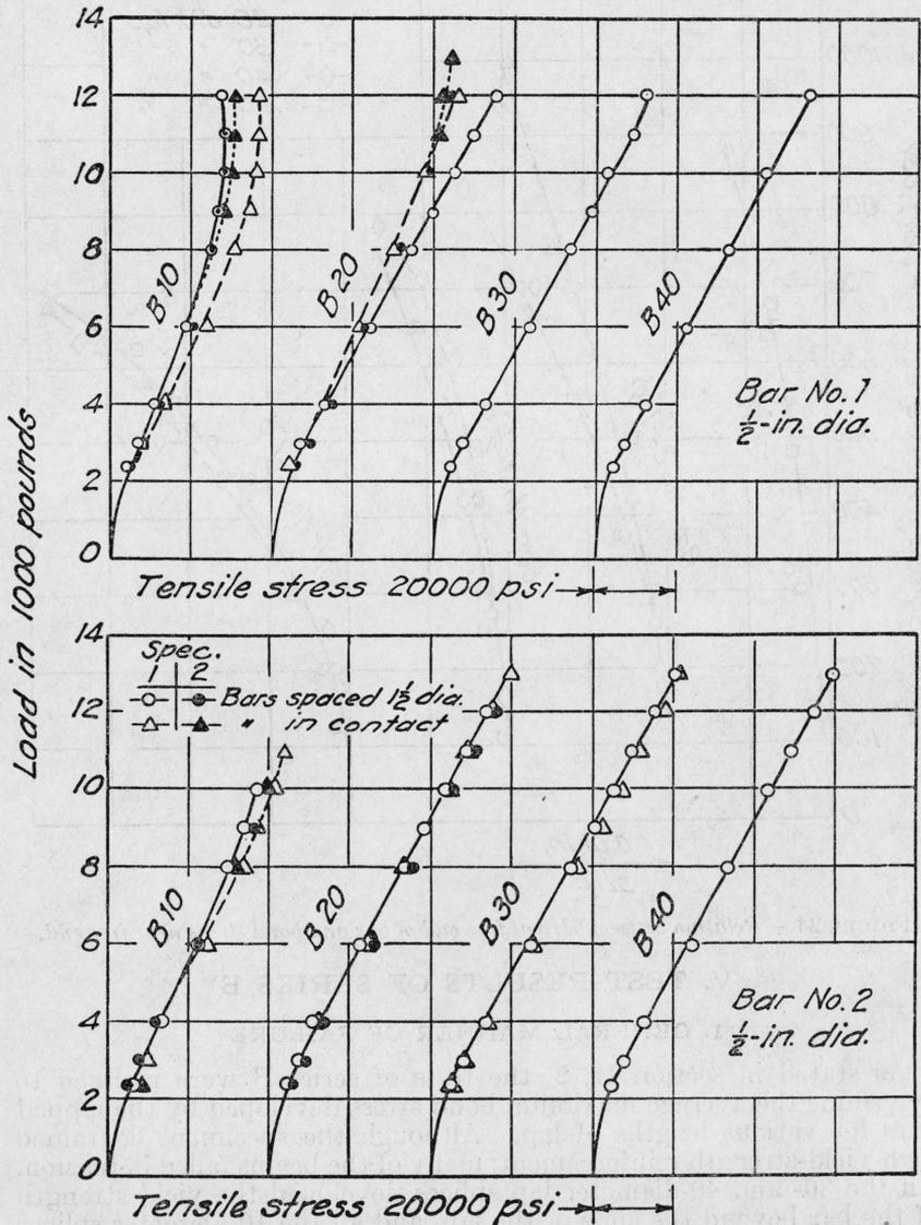
FIGURE 25.—Load-stress relation for lapped bars outside limits of splice.
