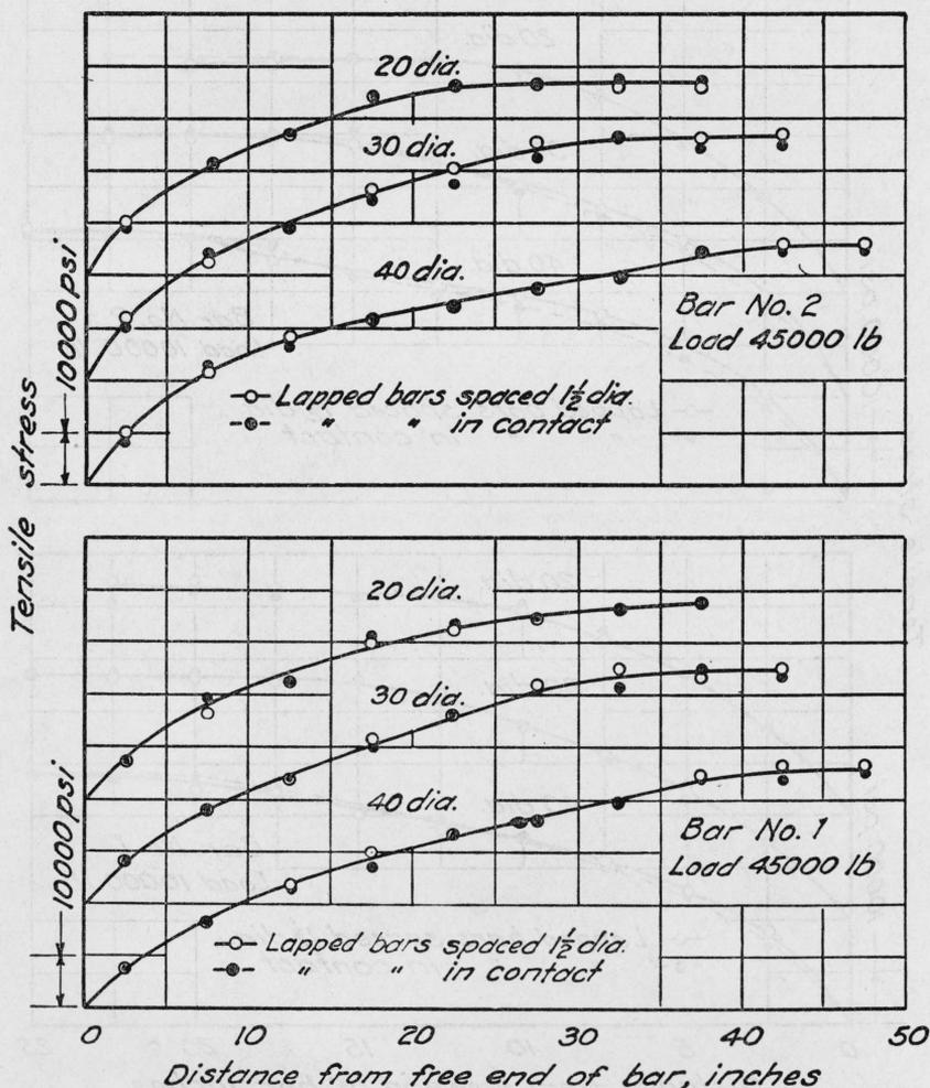
FIGURE 21.—Distribution of stress along lapped bars of two types of lap-splices. 1-in. bars. Stress values are the product of the modulus of elasticity and observed strains.
