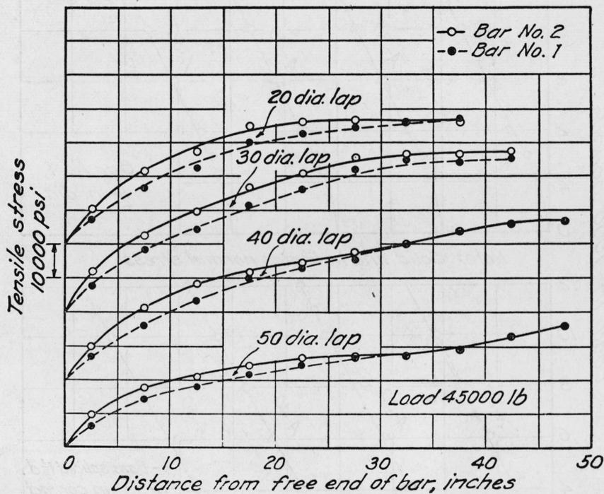
FIGURE 17.—Distribution of stress along lapped bars compared for No. 2 and No. 1 1-in. bars.
