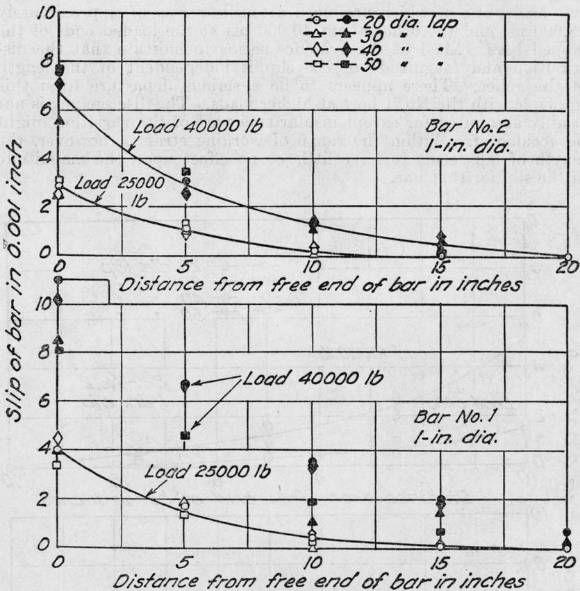
FIGURE 23.—Distribution of slip along lapped 1-in. bars.
