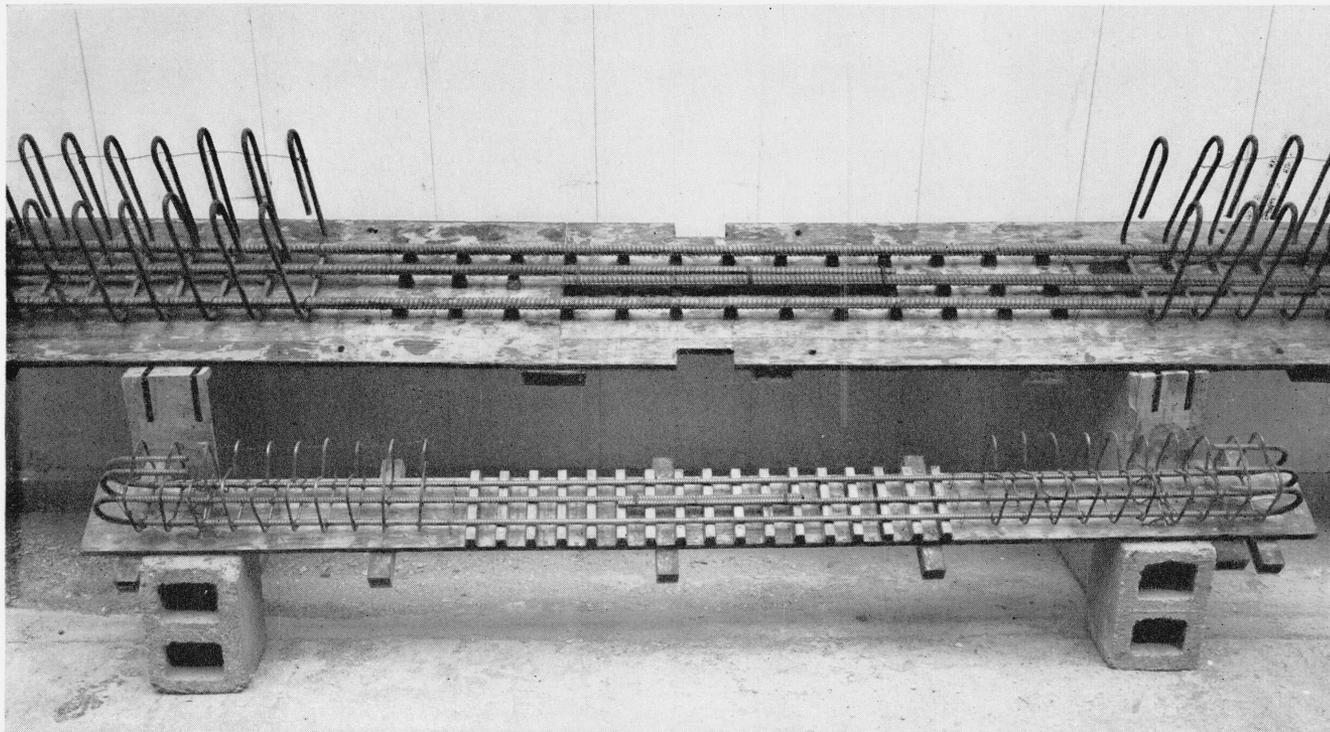
FIGURE 2.—*Reinforcement for 30-bar diameter splice.*
