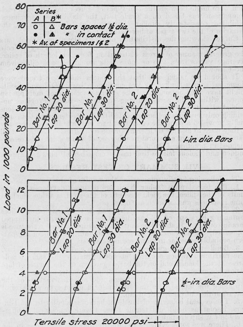
FIGURE 27.—Comparison between load-stress diagrams of series A and series B. Stress outside limits of splice. Stress values are the product of the modulus of elasticity and observed strains.
