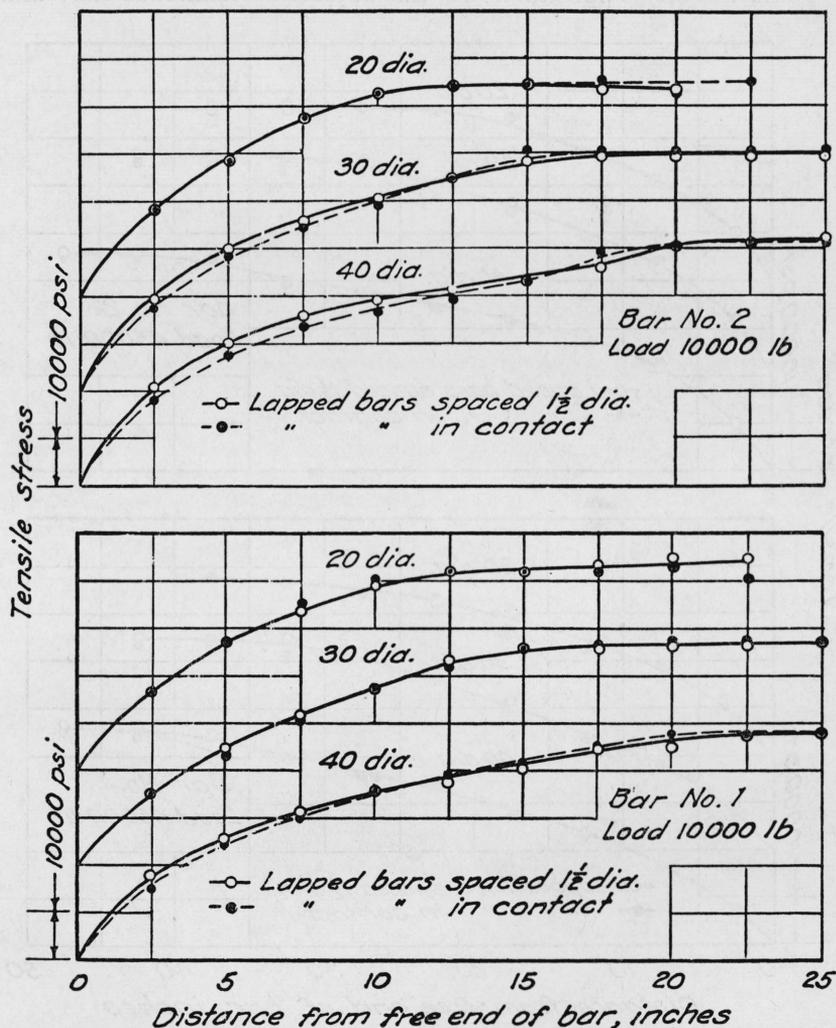
FIGURE 20.—Distribution of stress along the lapped bars of two types of lap-splices.  $\frac{1}{2}$ -in. bars. Stress values are the product of the modulus of elasticity and observed strains.
