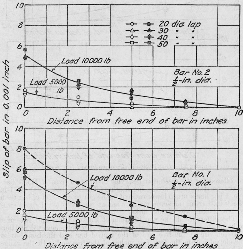
FIGURE 22.—Distribution of slip along lapped  $\frac{1}{2}$ -in. bars.
