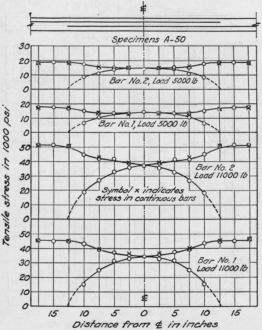
FIGURE 9.—Distribution of stress along lapped bars.
