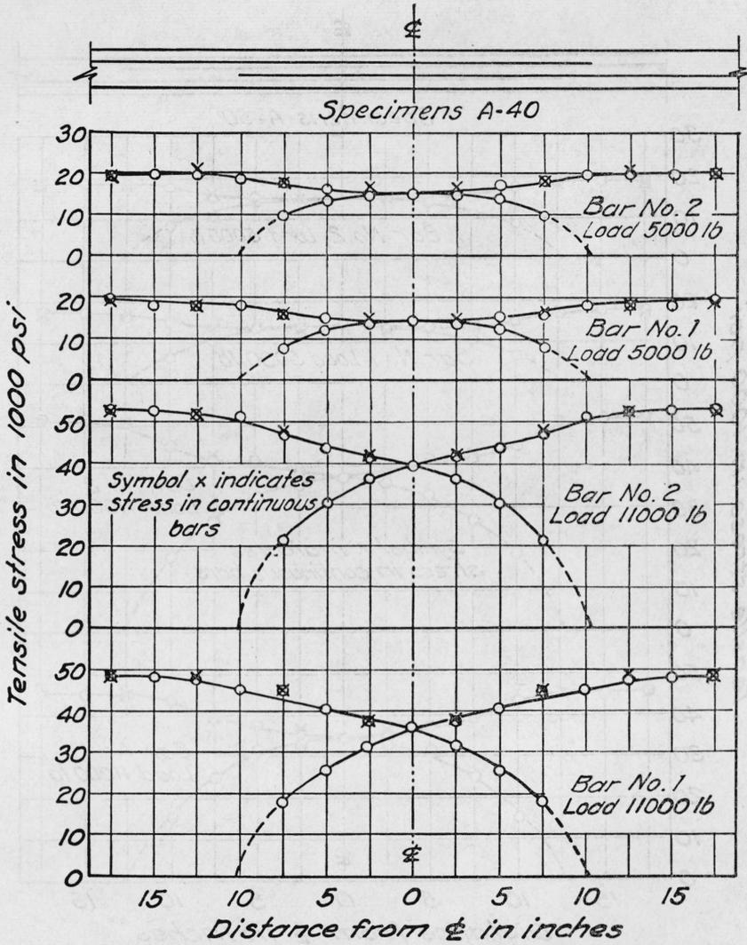
FIGURE 8.—Distribution of stress along lapped bars.
