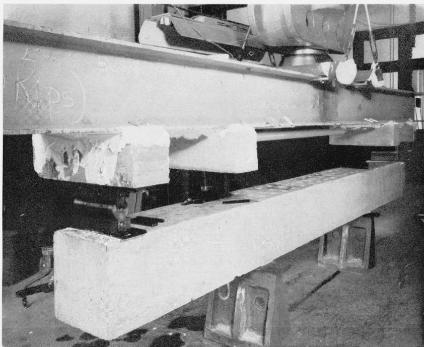
FIGURE 4.—Twelve-foot beam of series A under load.
