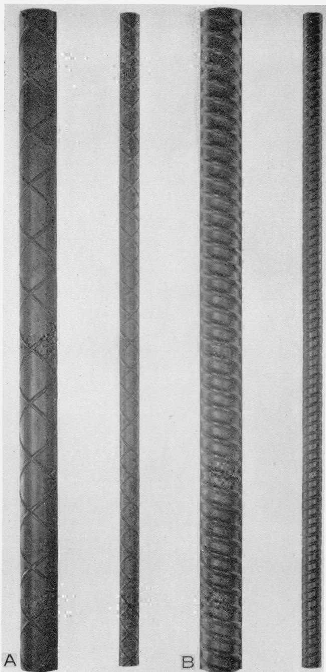
FIGURE 1.—*Reinforcing bars.*
