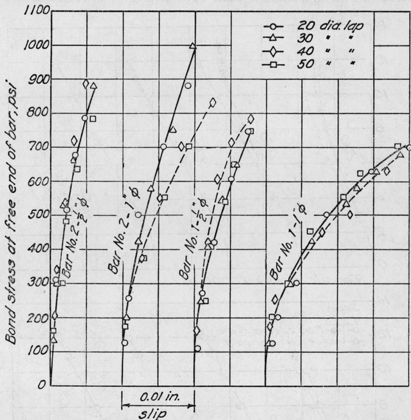
FIGURE 24.—Relation between slip at free end of bar and bond stress near free end.
