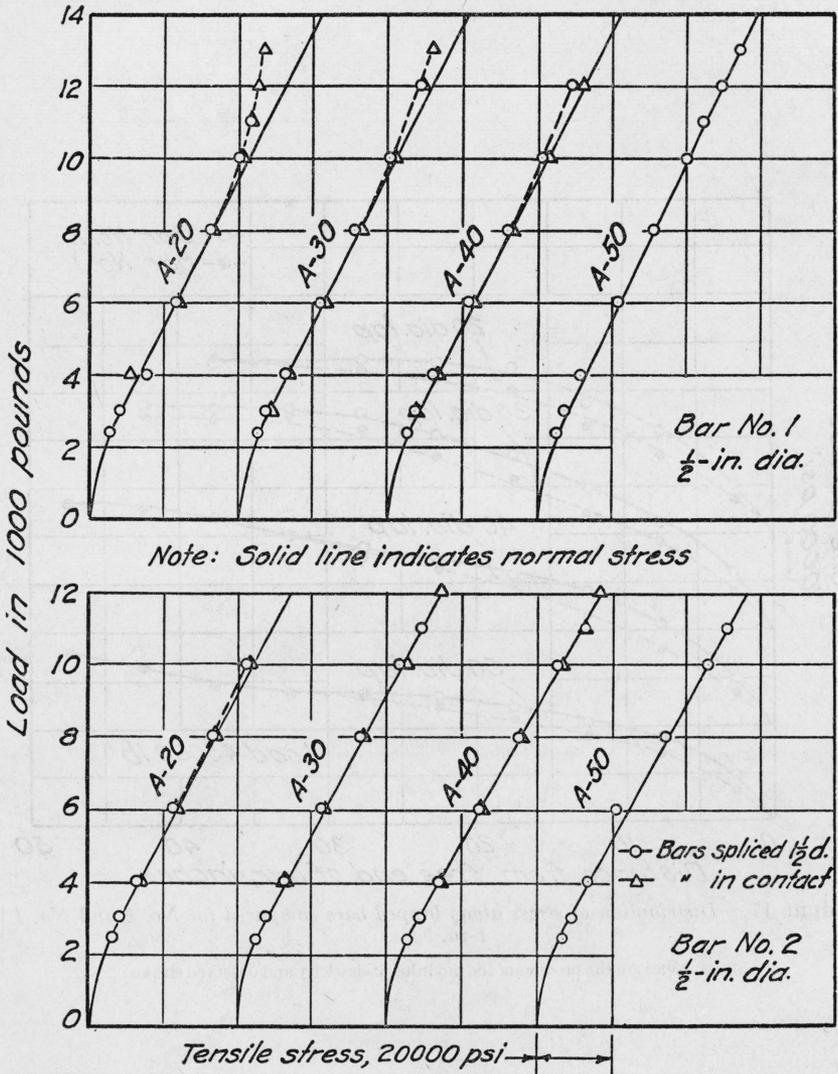
FIGURE 18.—Load-stress relation for lapped bars at limits of the splice.
