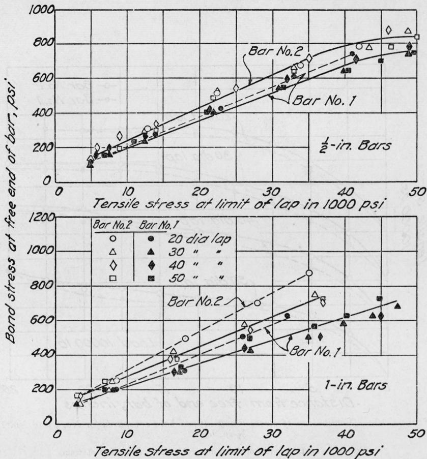
FIGURE 15.—Relation between bond stress at free end of bar and tensile stress at limit of lap.
