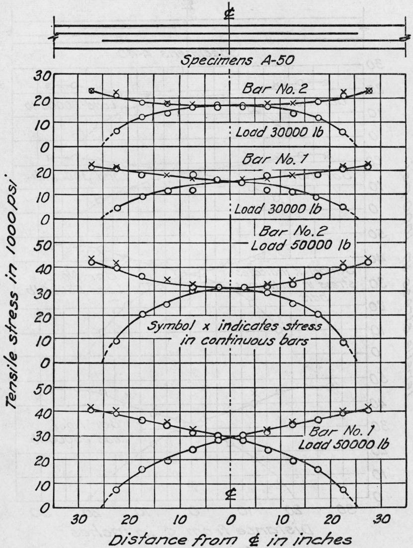
FIGURE 13.—Distribution of stress along lapped bars.
