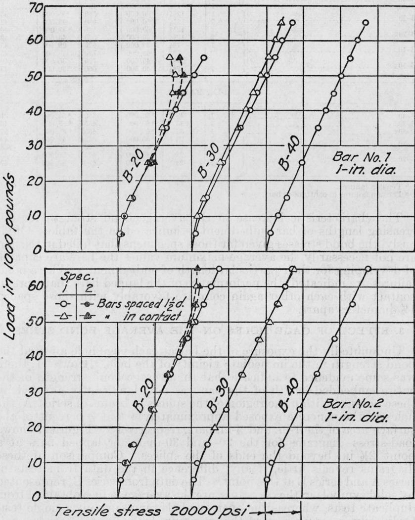
FIGURE 26.—Load-stress relation for lapped bars outside limits of splice.
