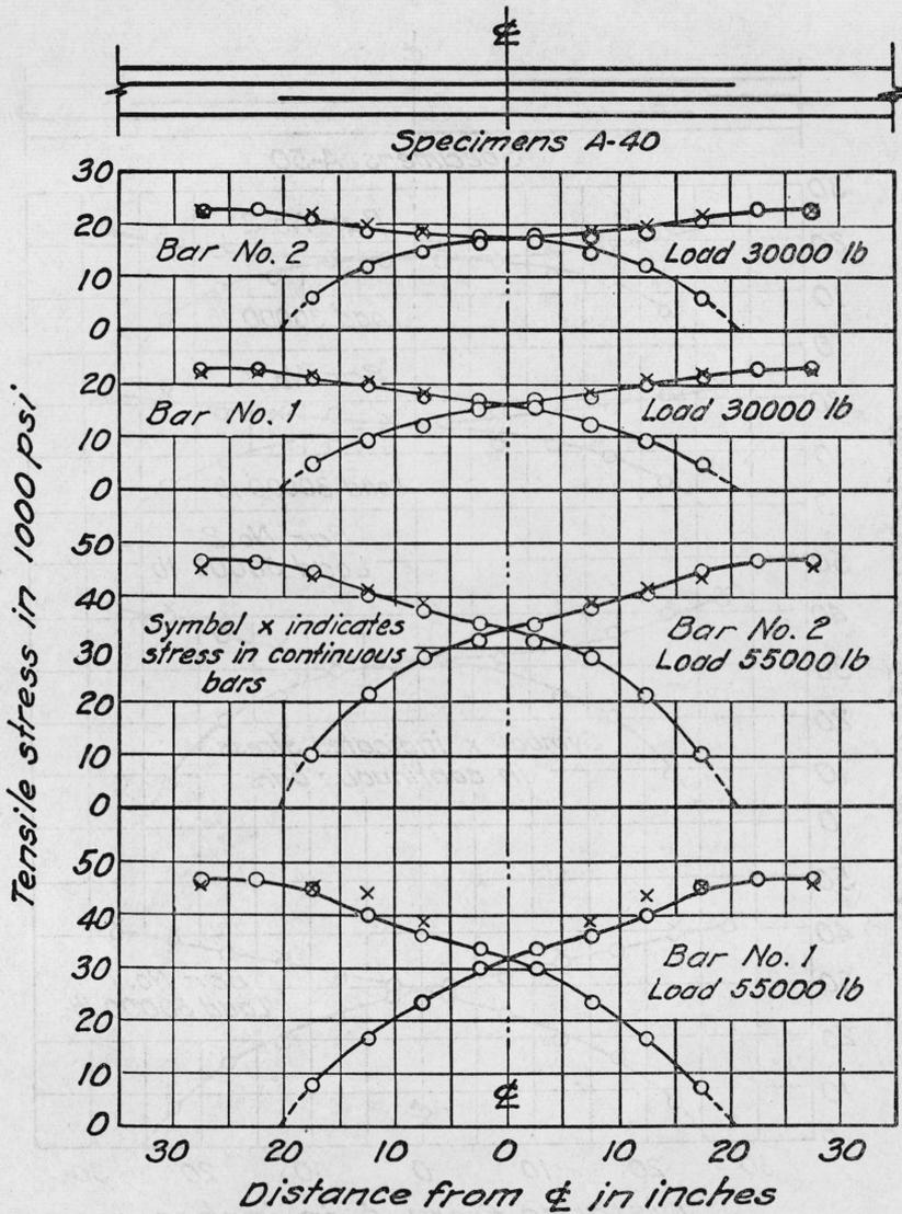
FIGURE 12.—Distribution of stress along lapped bars.
