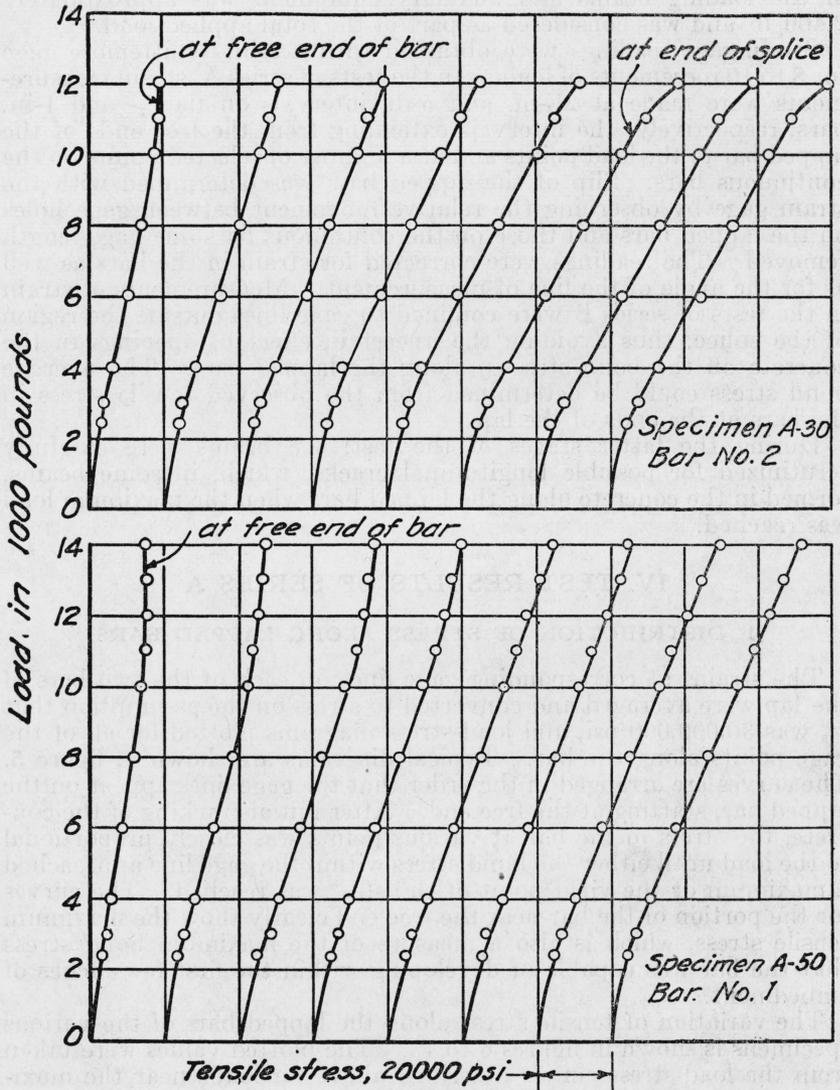
FIGURE 5.—Typical load-stress curves for successive gage lines along lapped bars.
