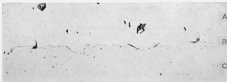
FIGURE 1.— Photomicrographic cross section perpendicular to direction of polishing, \times 500 .
