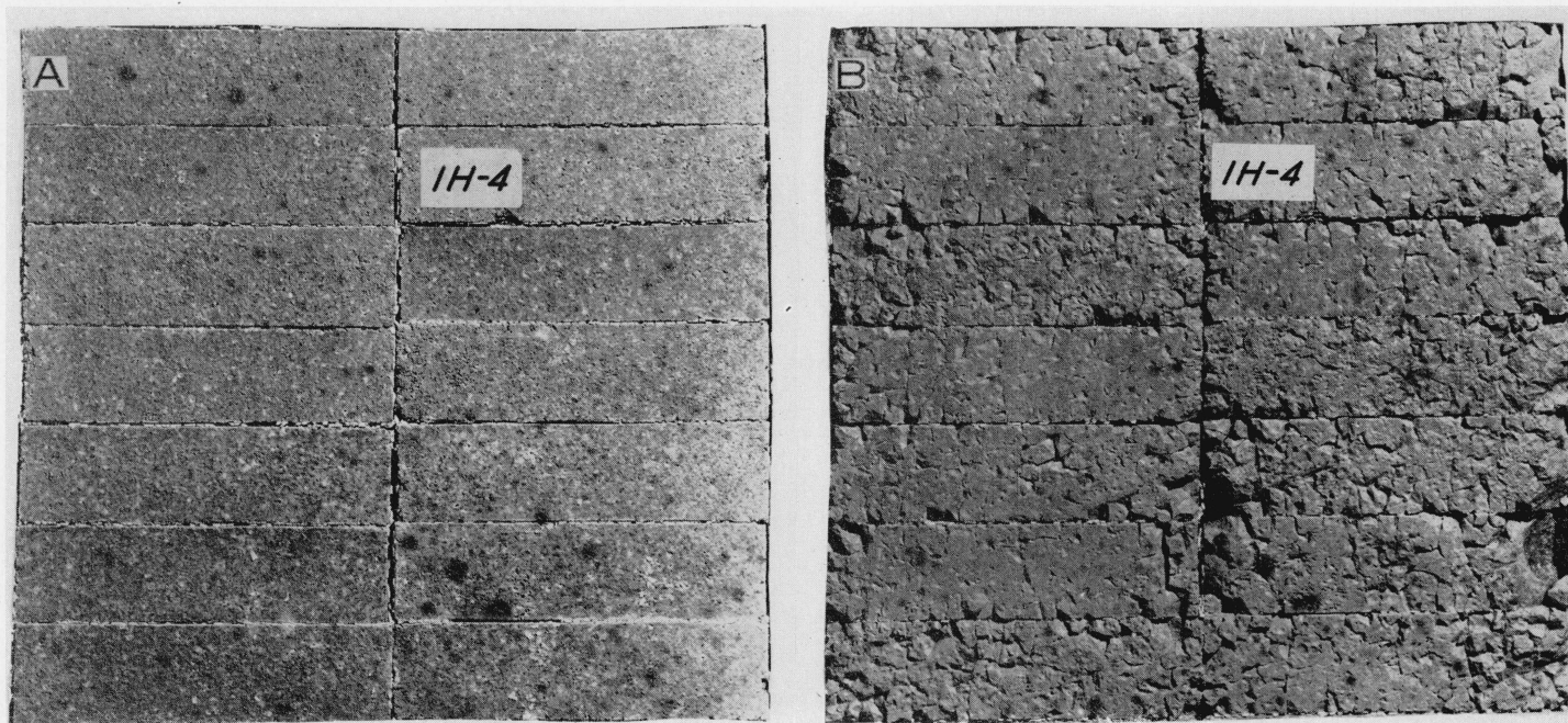
FIGURE 18.—Brand IH-4, A, after the preheating at 1,600° C; B, after the spalling test.
