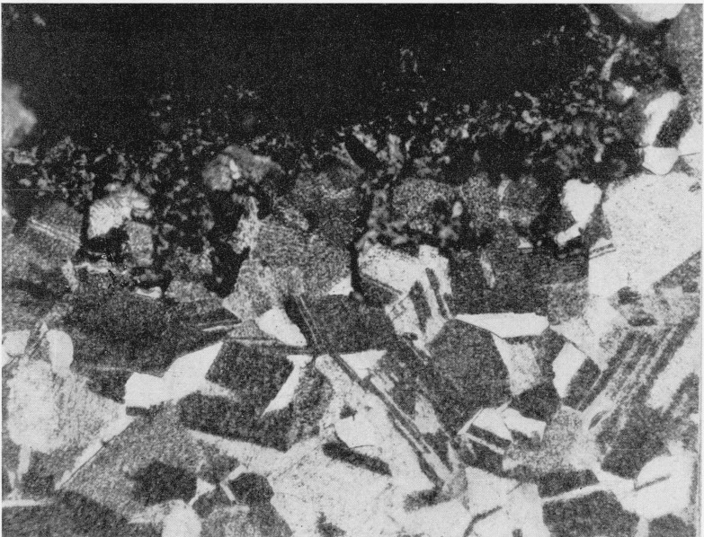
FIGURE 12.— Admiralty metal exposed 9.53 years to Sharkey clay. Transverse section to show thin layer dezincified metal. \times 500 .
