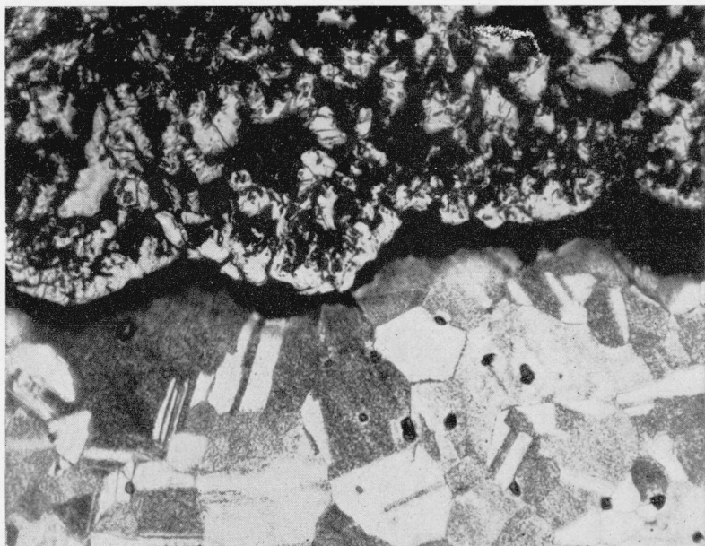
FIGURE 9.— Yellow brass exposed 9.53 years to Sharkey clay. Transverse section showing uncorroded metal (below) and dezincified metal (above). \times 500 .
