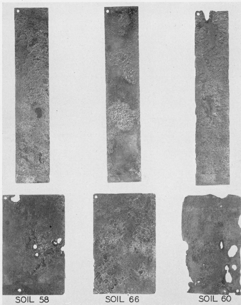
FIGURE 15.—Rolled (above) and die-cast (below) zinc buried in muck (soil 58), in Mohave fine gravelly loam (soil 66), and in Rifle peat (soil 60), approximately 4 years each.
