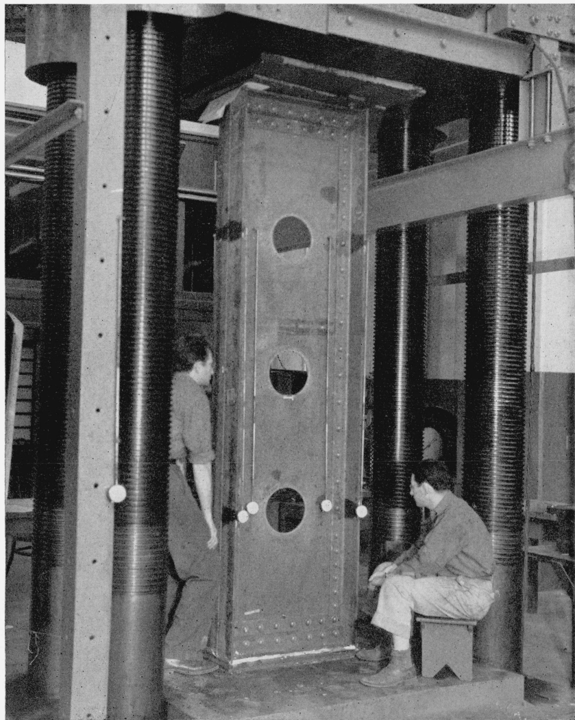
FIGURE 2.—Column C6A in the testing machine during the test in elastic range.
