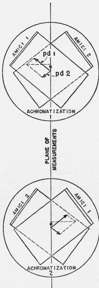
FIGURE 2.—Effect of principal plane deviation ( $pd$ ) by Amici prisms.
