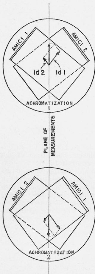
FIGURE 1.—Effect of lateral deviation ( $ld$ ) by Amici prisms.
