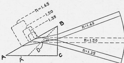
FIGURE 4.—Mounting of refractometer block with respect to axis of rotation.
