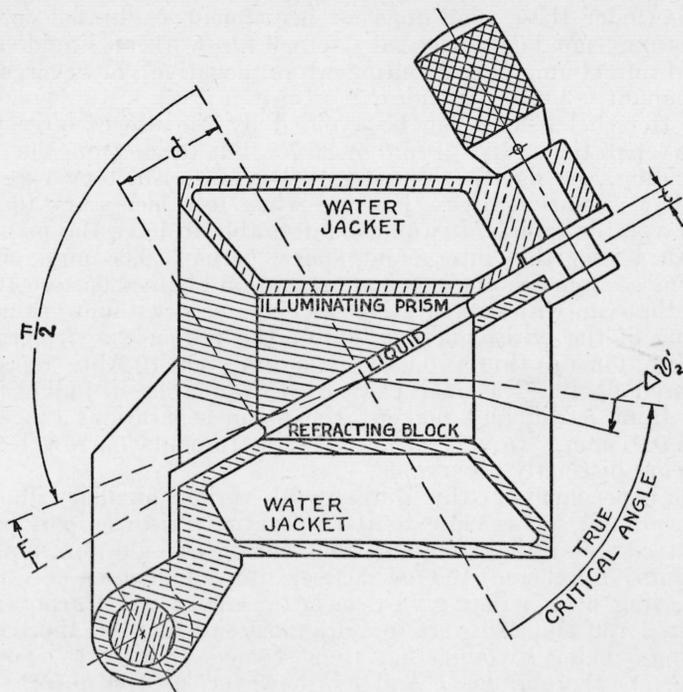
FIGURE 6.—Geometrical shielding of critical rays caused by separation of Abbe prisms.
