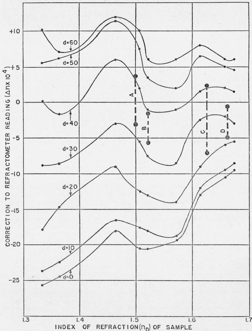
FIGURE 3.—Calibration curves for refractometer having a defective compensator.
