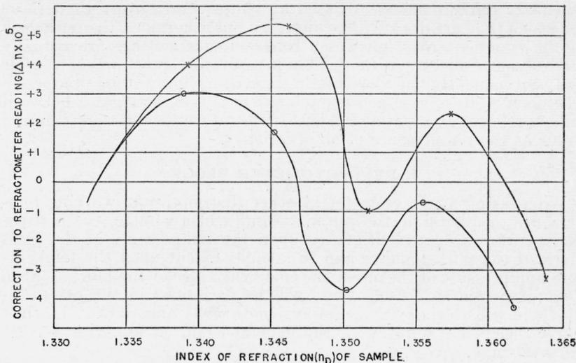
FIGURE 5.—Correction curves showing the systematic nature of small errors in performance of very good dipping refractometers.
