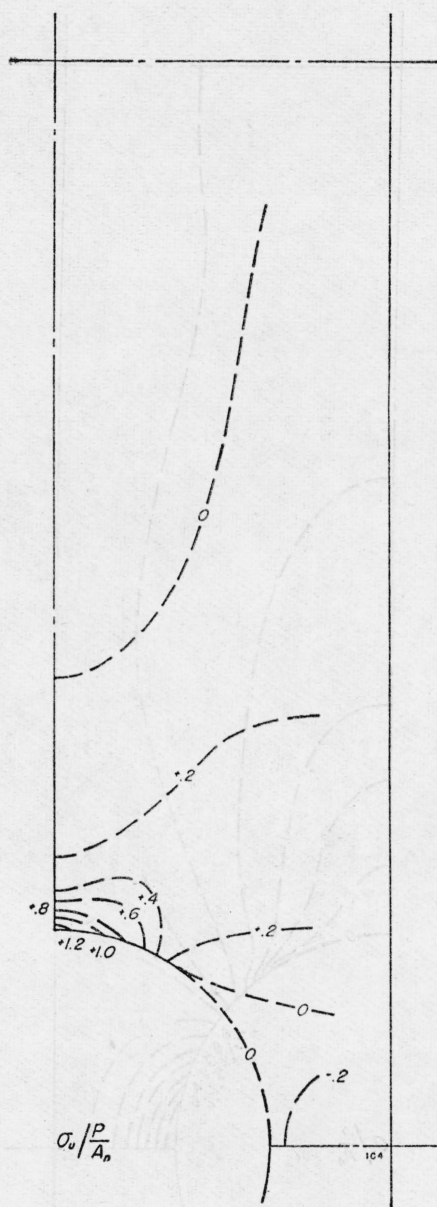
FIGURE 13.—Column C1C (2-3) (four angles), perforation spacing .45 inches. Isogram of maximum principal stress.
