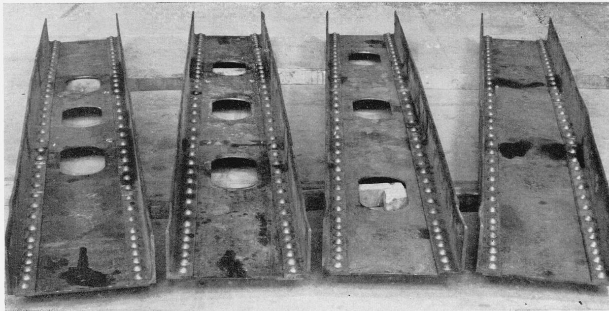
FIGURE 19.—Columns C3—(two angles) after maximum load tests.
