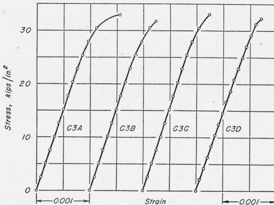
FIGURE 17.—Columns C3—(two angles). Stress-strain graphs.
