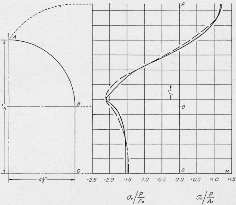
FIGURE 4.—Columns C3C, perforation spacing 5 1/4 inches. Distribution of stress on the edge of the middle perforation.
