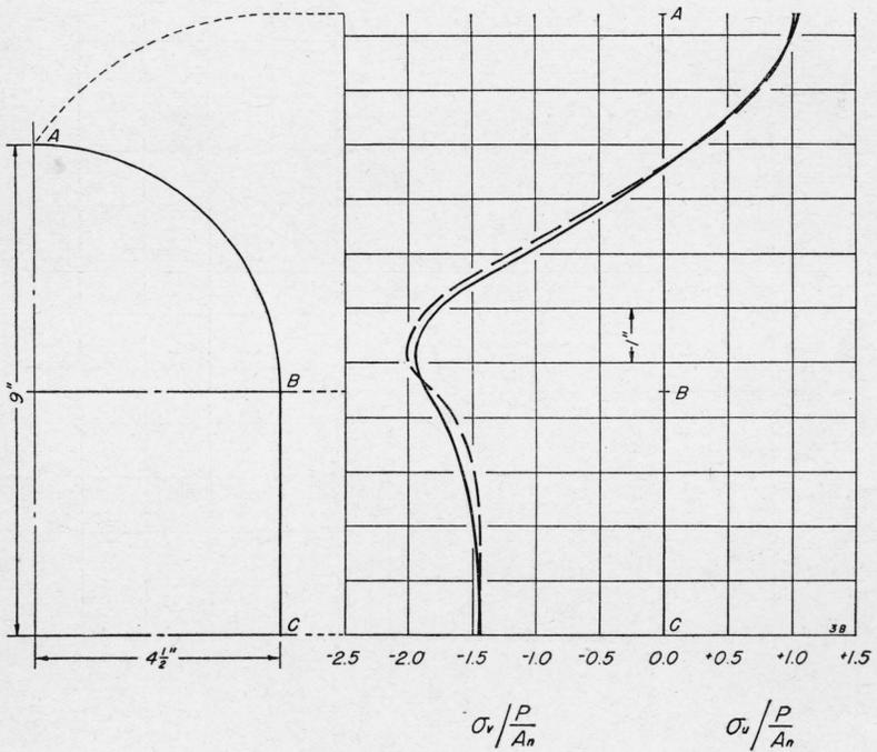
FIGURE 3.—Columns C3B, perforation spacing 42 inches. Distribution of stress on the edge of the middle perforation. The solid line is for the two-angle, and the dashed line for the four-angle, column. Based on net area.
