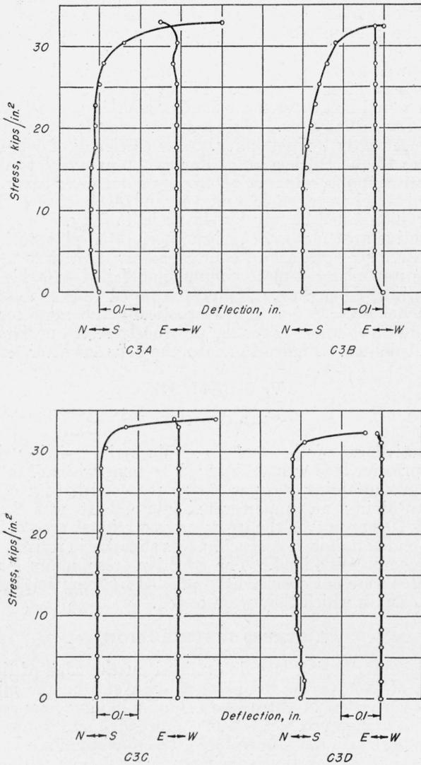
FIGURE 18.—Columns C3—(two angles). Stress-deflection graphs.
