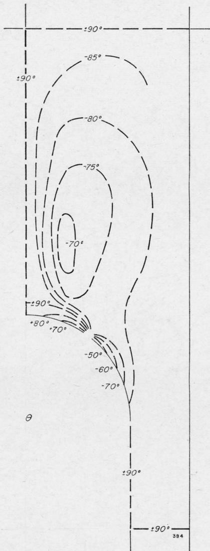
FIGURE 11.—Column C3B(2-3) (four angles), perforation spacing 42 inches. Isoclines.
