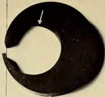
QUENCHED 5 TIMES IN WATER AT 70°C (CRACKED)
