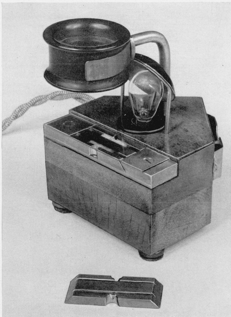
FIGURE 11.—Instrument for measuring the length of a tuft of pile.
