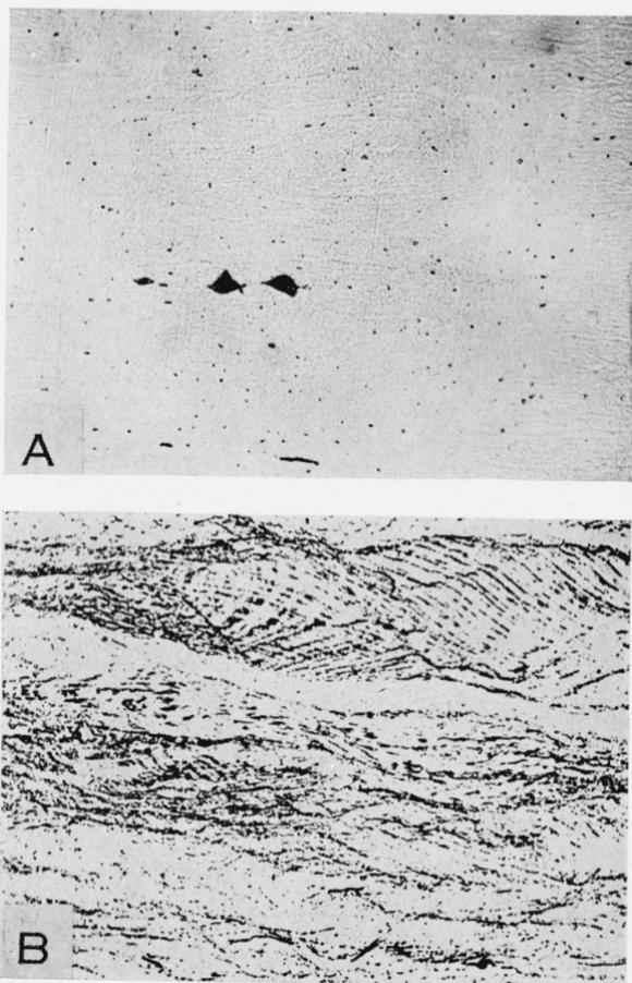
FIGURE 11.—18-8 (material *E*), microstructure of specimens heated 30 minutes at: A, 900° F.; B, 1,000° F.  $\times 500$ .
