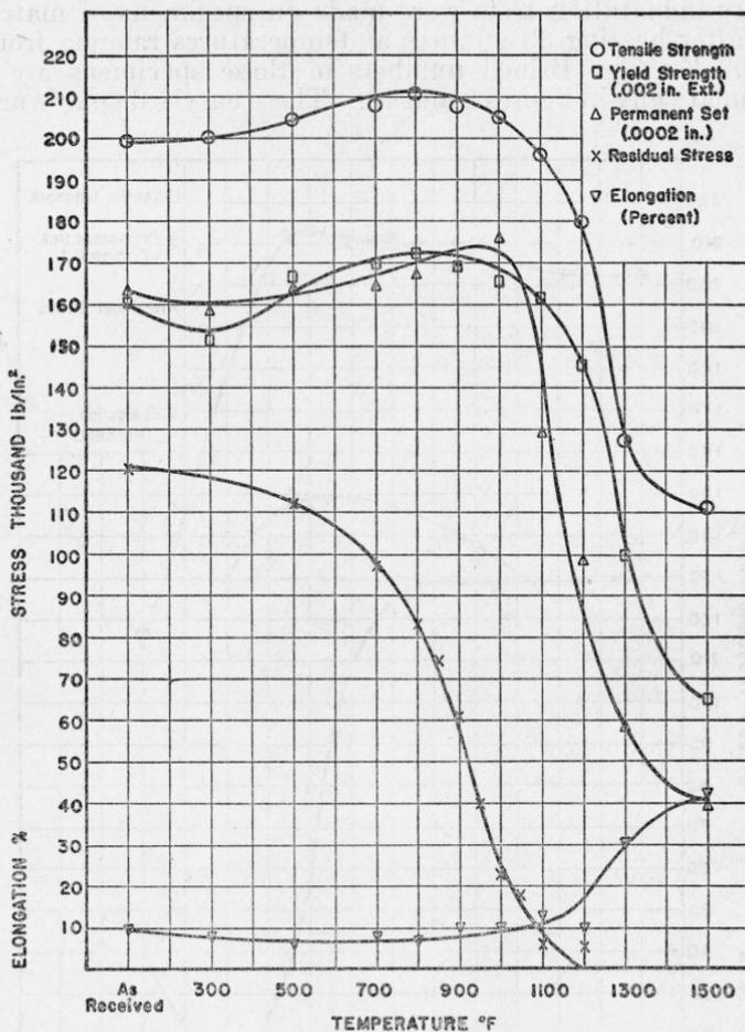
FIGURE 7.—18-8-Cb (material K), effect of heat treatment on physical properties and relief of residual stress.
