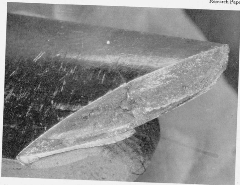
FIGURE 1.—*Torsional fatigue fracture in 18-8 stainless steel tierod;  $\times 5$ .*
