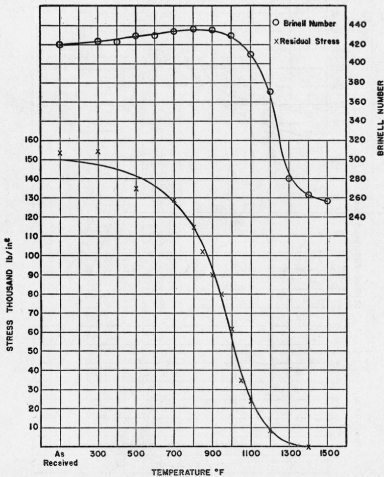
FIGURE 9.—18-8 (material E), effect of heat treatment on Brinell number and relief of residual stress.
