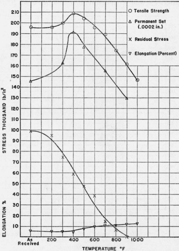
FIGURE 3.—SAE 1050 steel (material A), effect of heat treatment on physical properties and relief of residual stress.
