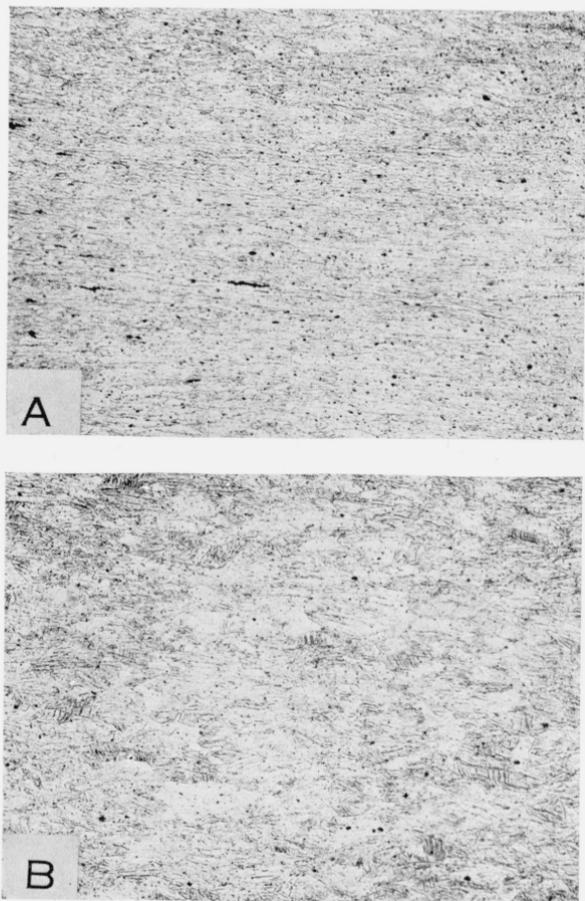
FIGURE 13.—*A, microstructure within X-band; B, microstructure outside X-band.*
