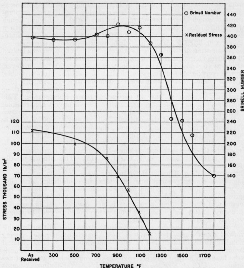
FIGURE 10.—18-8-Mo (material M), effect of heat treatment on Brinell number and relief of stress.
