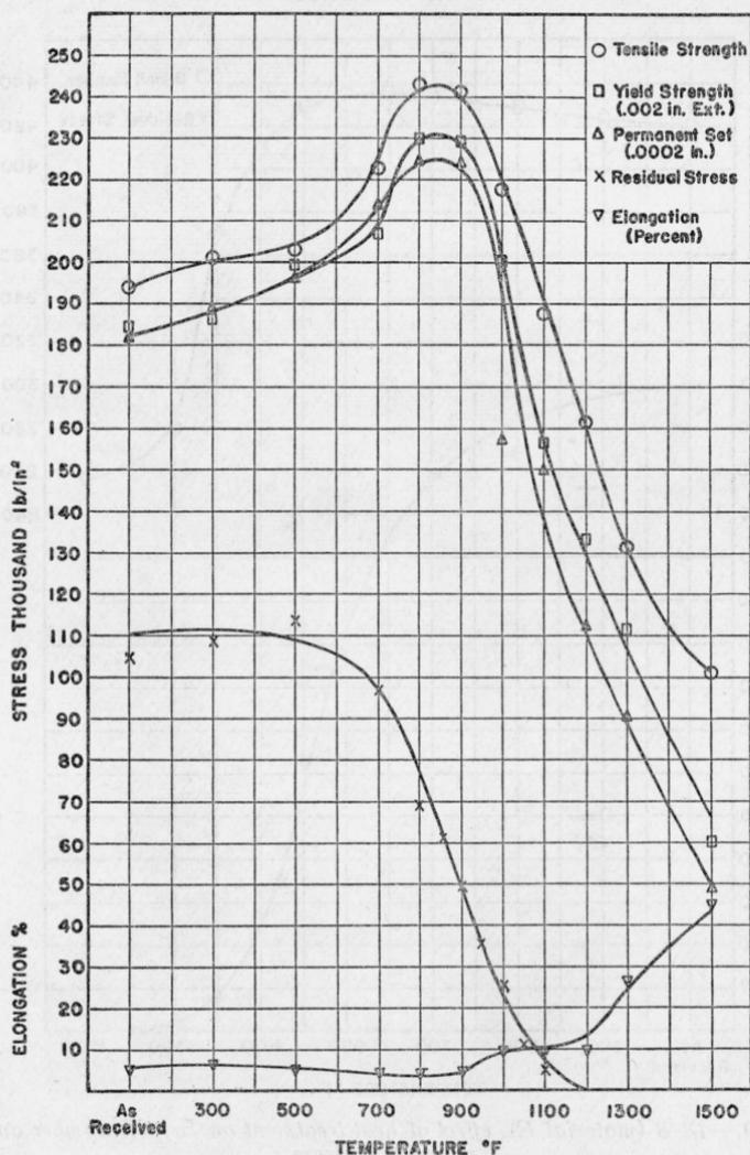
FIGURE 8.—18-8-Ti (material *H*), effect of heat treatment on physical properties and relief of residual stress.
