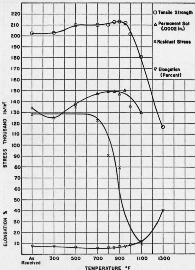
FIGURE 6.—18-8 (material *C*), effect of heat treatment on physical properties and relief of residual stress.
