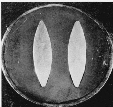
FIGURE 12.—*X-bands in transverse sections of 18-8 titanium rods.*
