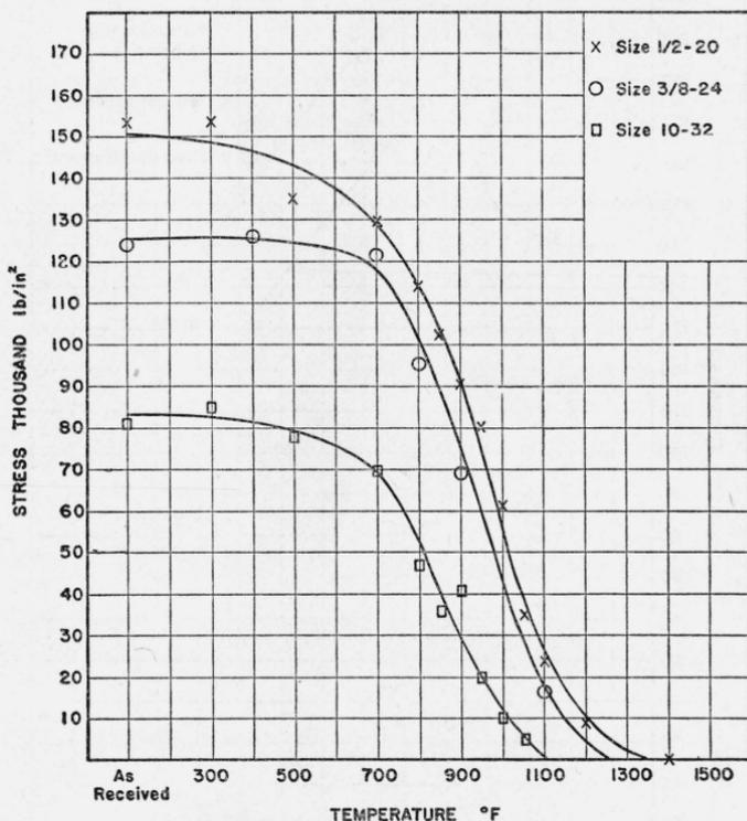
FIGURE 4.—18-8 (materials *C*, *E*, and *F*), effect of heat treatment on relief of stress in tie-rods of different sizes.
