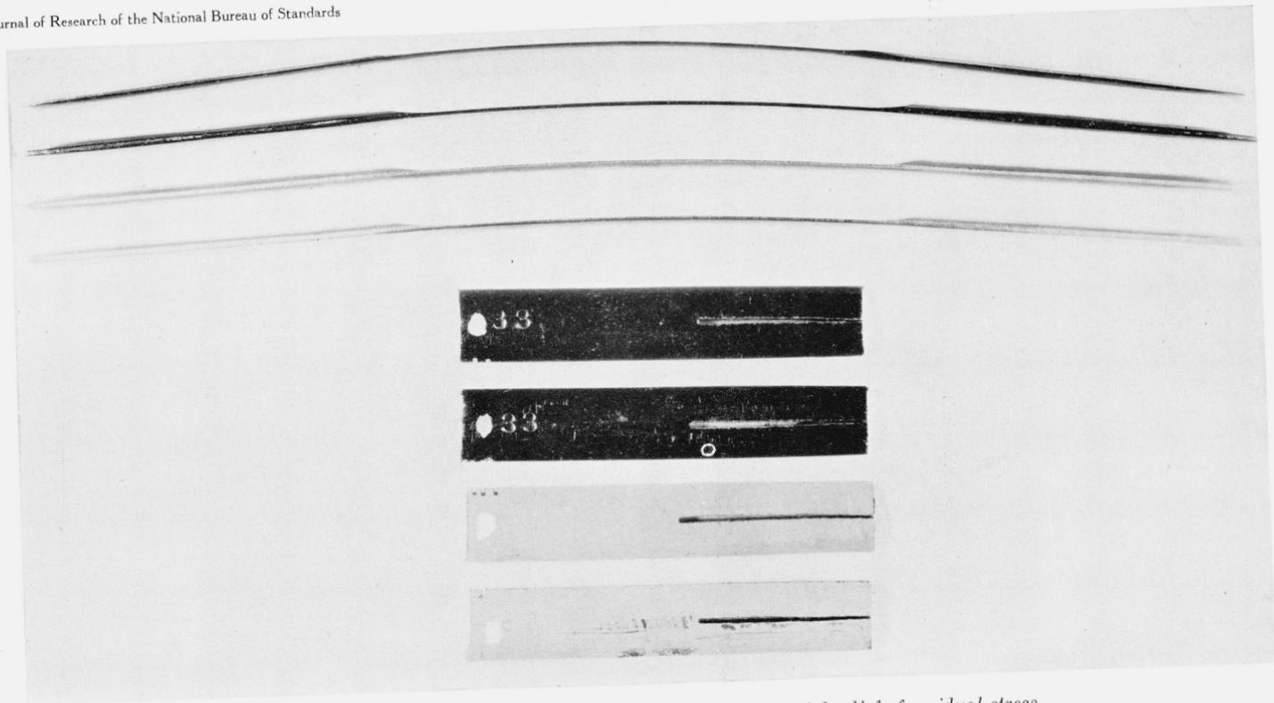
FIGURE 2.—*Distortion in tierod specimens caused by partial relief of residual stress.*
