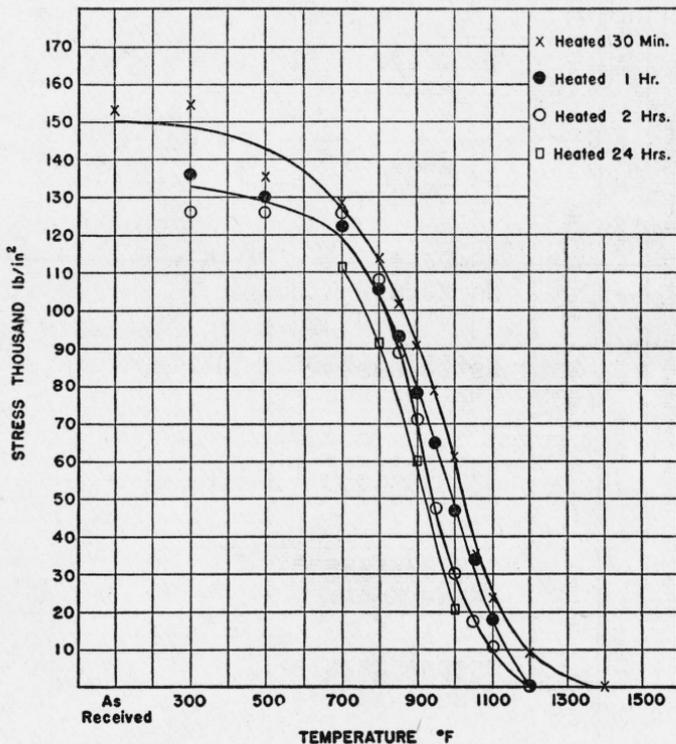
FIGURE 5.—18-8 (material E), effect of temperature and period of heating on relief of residual stress.
