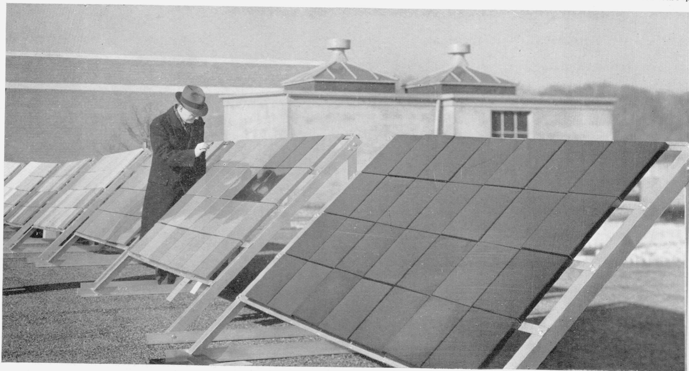
FIGURE 1.— Specimens in racks as exposed on a roof at the National Bureau of Standards, Washington, D. C.
