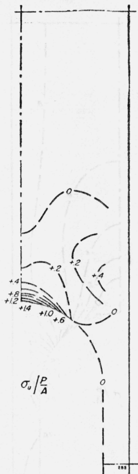
FIGURE 13.—Column C2B (2-3) (two angles). Isogram of maximum principal stress.
