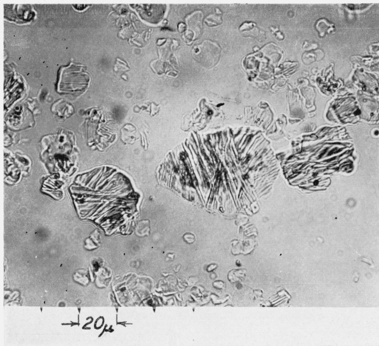
FIGURE 2.—Crystals having the probable formula K_2O \cdot 23CaO \cdot 12SiO_2 . Ordinary transmitted light.
