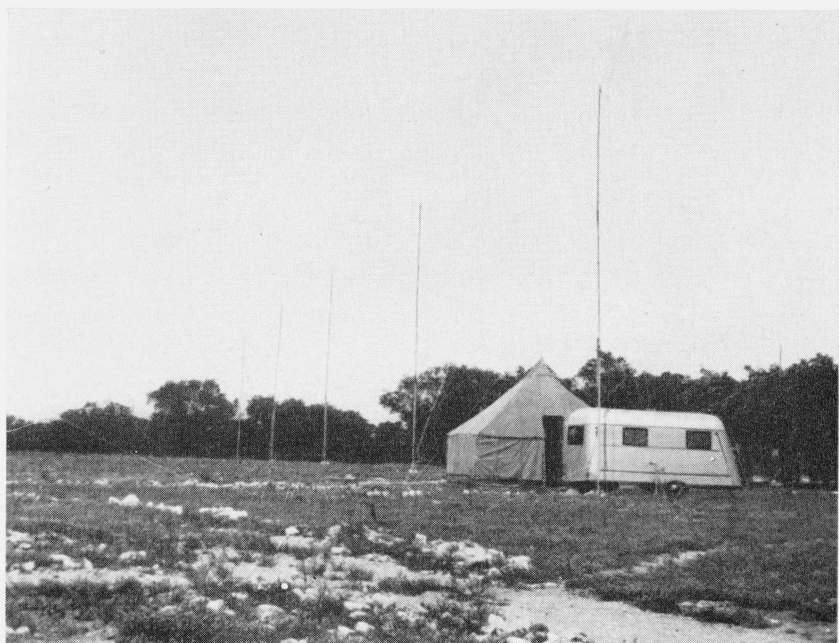
FIGURE 6.— Equipment as installed in the field, showing arrangement of bamboo masts and antennas.
