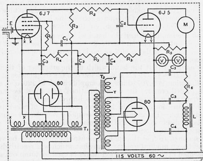
FIGURE 2.—Wiring diagram of output circuit and meter having the following circuit constants:
