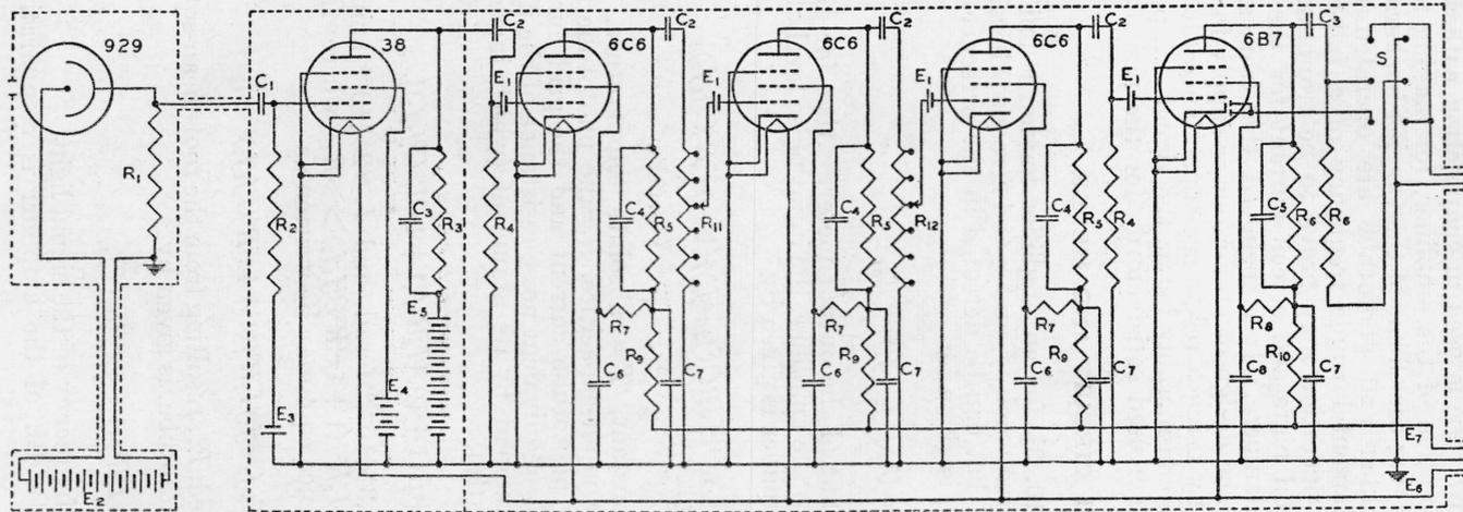
FIGURE 1.—Wiring diagram of phototube and 120-cycle, resistance, capacitance tuned amplifier having the following circuit constants:
