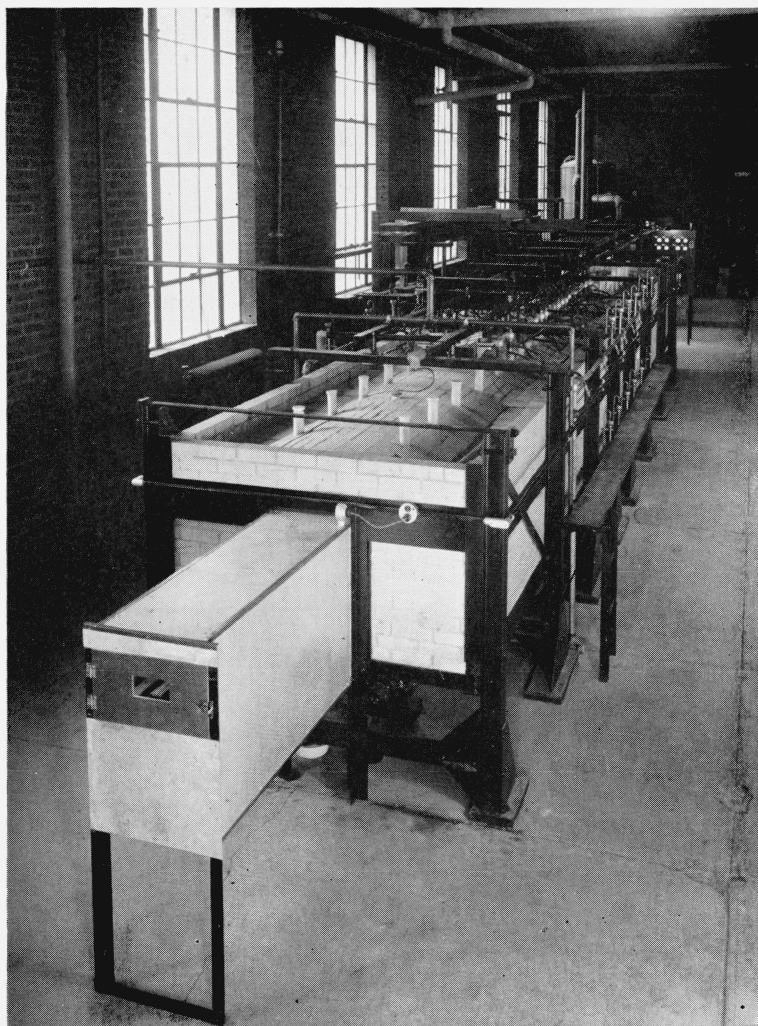
FIGURE 3.— Electrically heated tunnel kiln.
