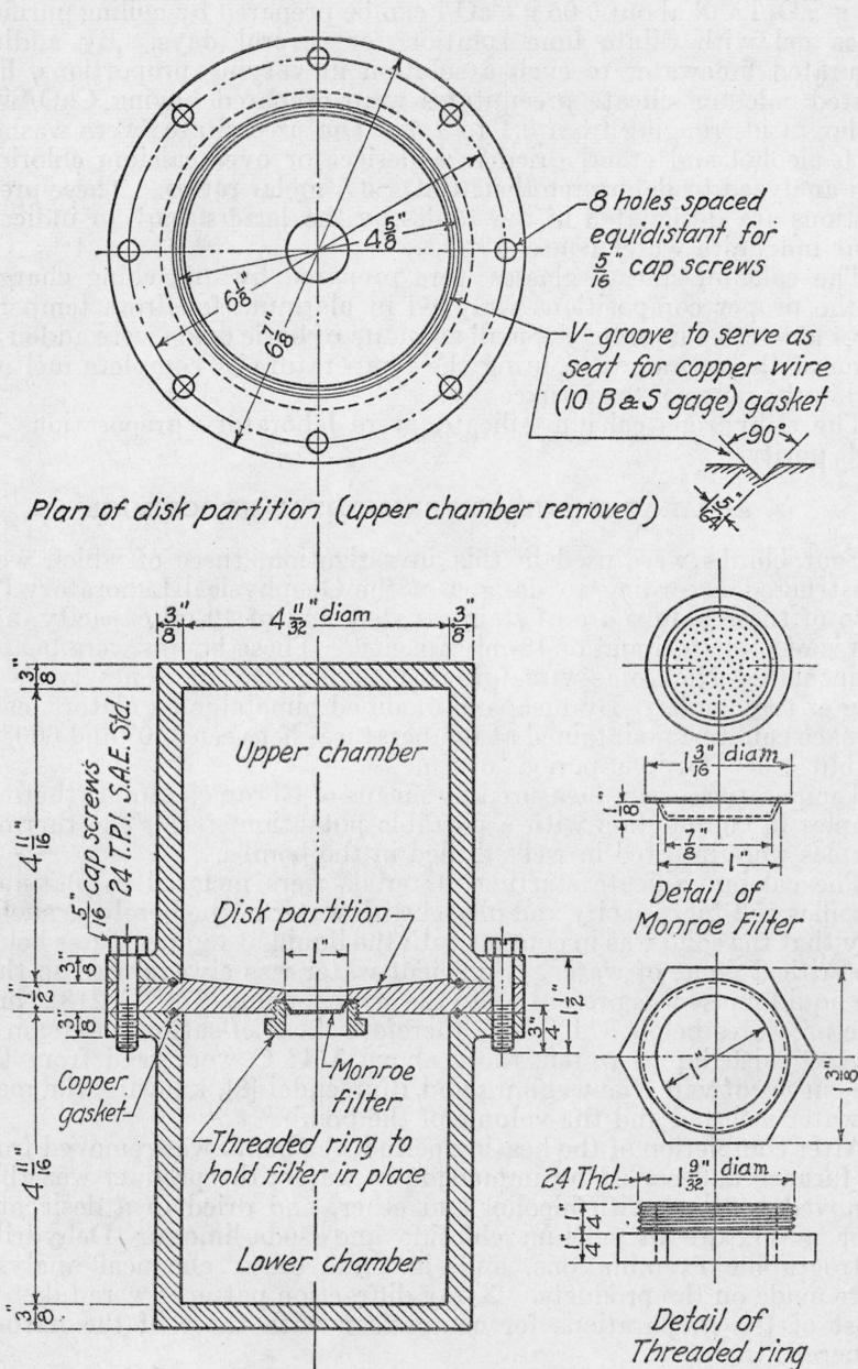
FIGURE 1.—Bomb for hydrothermal synthesis (in position for filtering).
