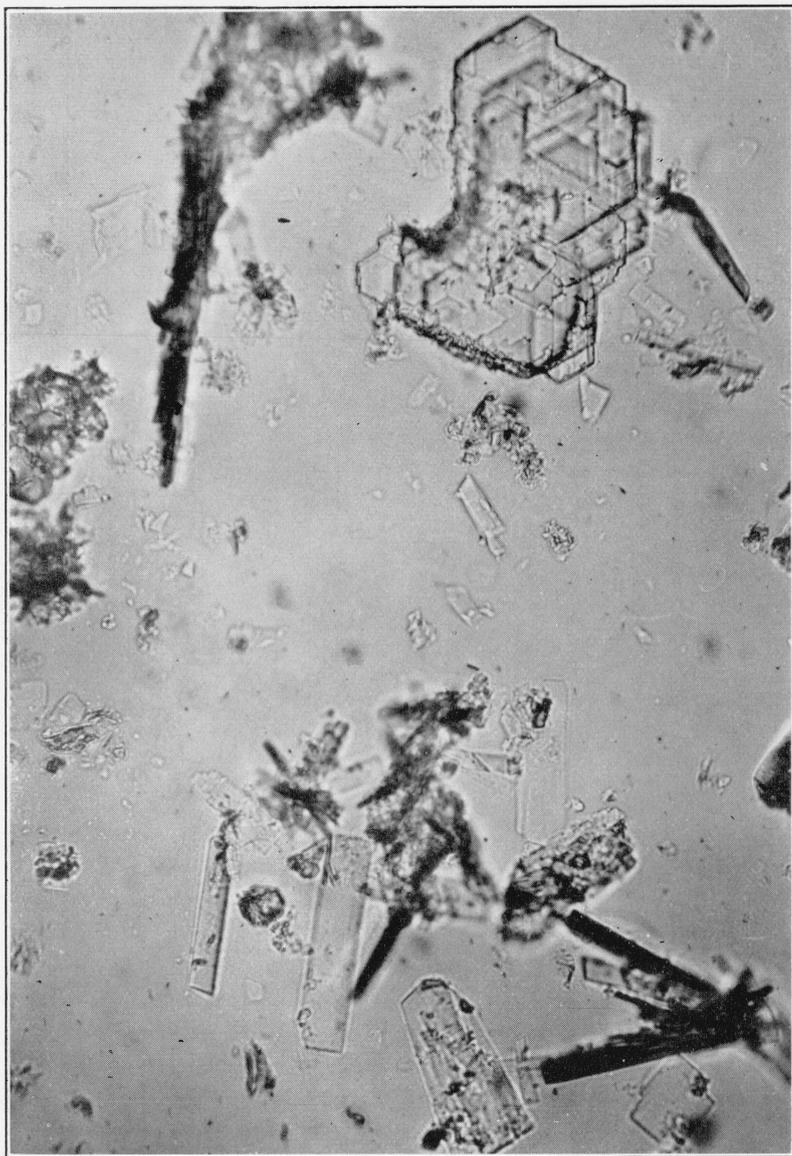
FIGURE 10.—Lath-like orthorhombic plates of synthetic  $10\text{CaO}\cdot 5\text{SiO}_2\cdot 6\text{H}_2\text{O}$  and hexagonal plates of  $\text{Ca}(\text{OH})_2$  obtained by treatment of portland cement clinker with water at  $175^\circ\text{C}$ .
