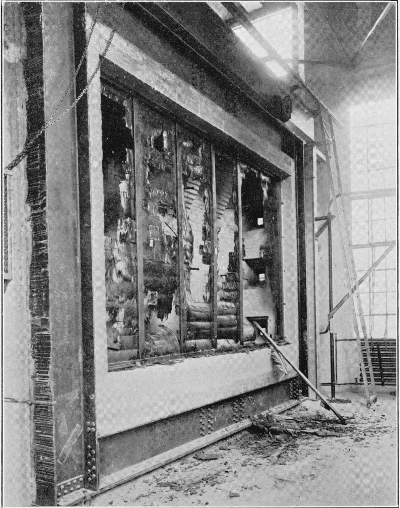
FIGURE 7.—Unexposed side of panel B after fire exposure.
