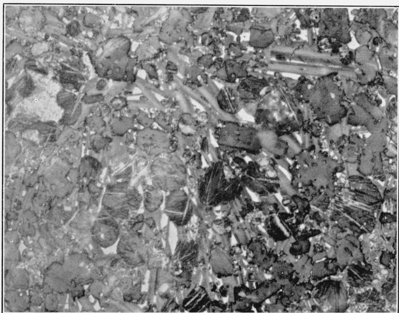
FIGURE 16.— Same field as figure 15, but etched with water for 2 seconds, followed by 1-percent \text{HNO}_3 in alcohol for 2 seconds.
