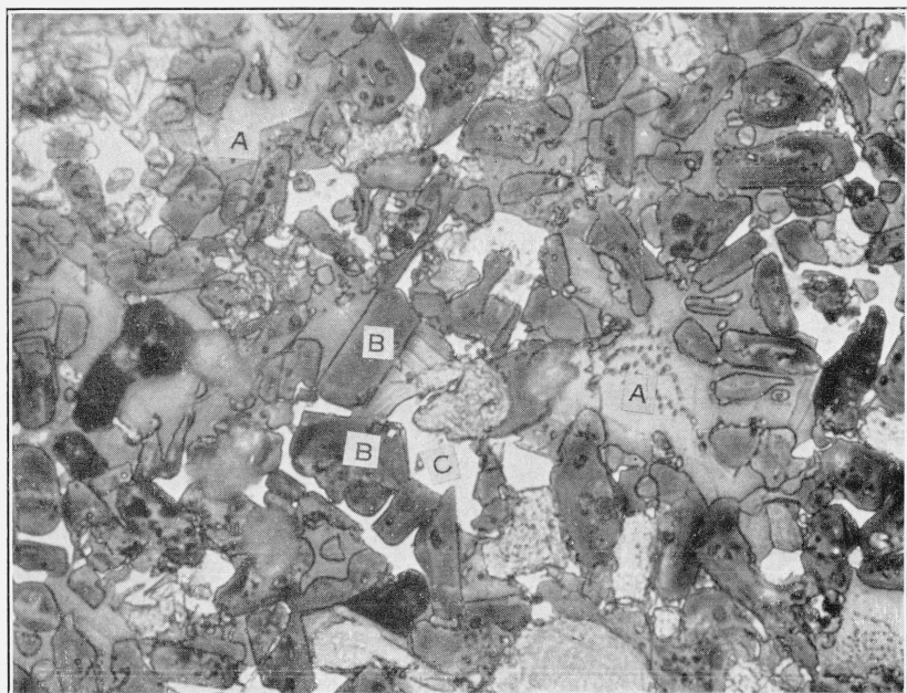
FIGURE 5.— Rectangular type of dark interstitial material in commercial cement clinker.
