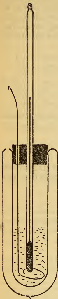
FIG. 13.—Apparatus for determining time-temperature cooling curves
