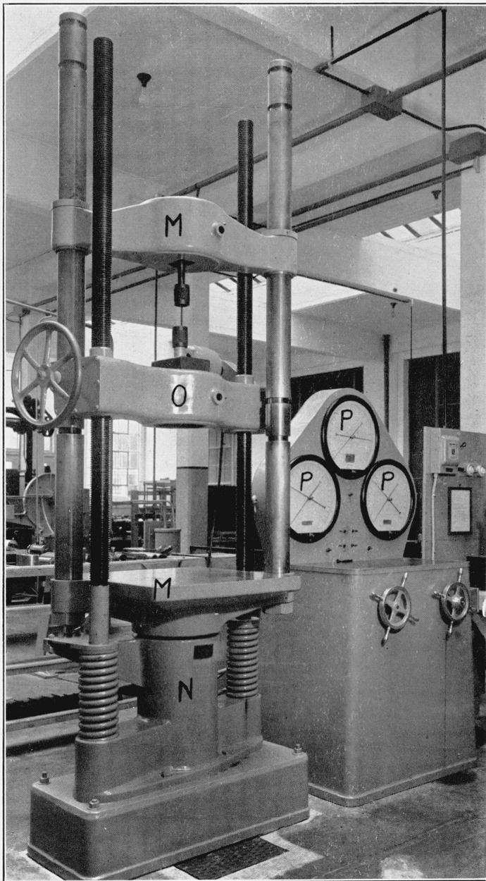
FIGURE 5.—Machine E, 100,000-pound capacity fluid-support, Bourdon-tube, hydraulic testing machine.
