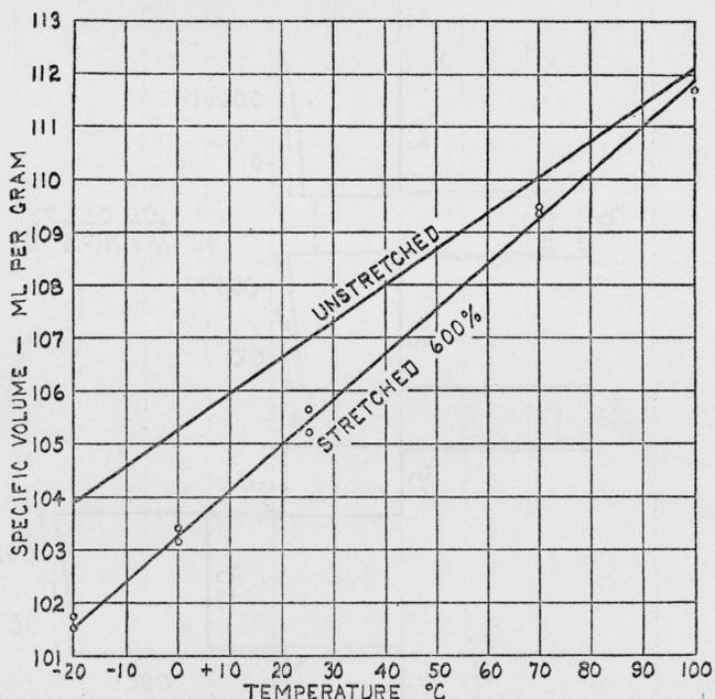
FIGURE 11.—Specific volume-temperature relations for unstretched rubber and rubber stretched to 600-percent elongation.
