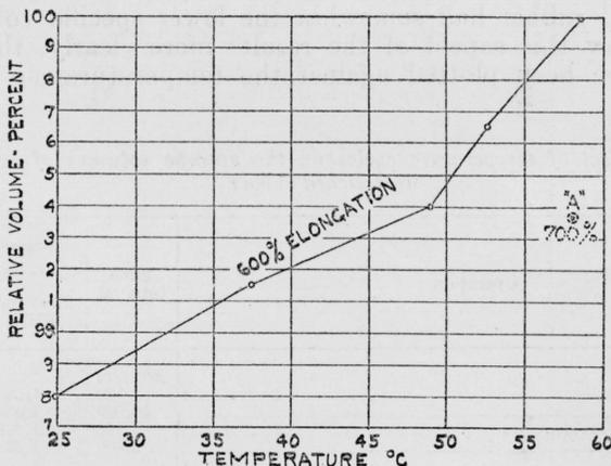
FIGURE 9.—Change in volume of rubber when stretched to 600-percent elongation and held for 3 minutes at different temperatures.
