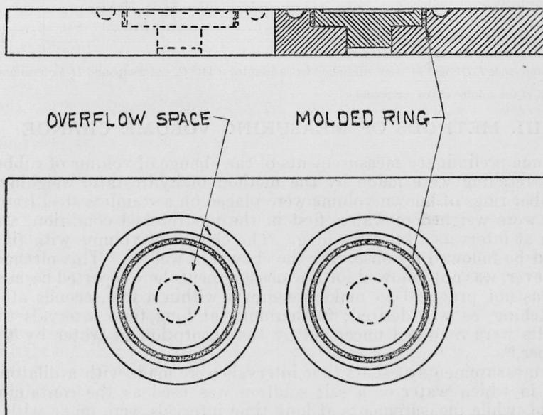
FIGURE 1.—Mold for rubber test rings.
