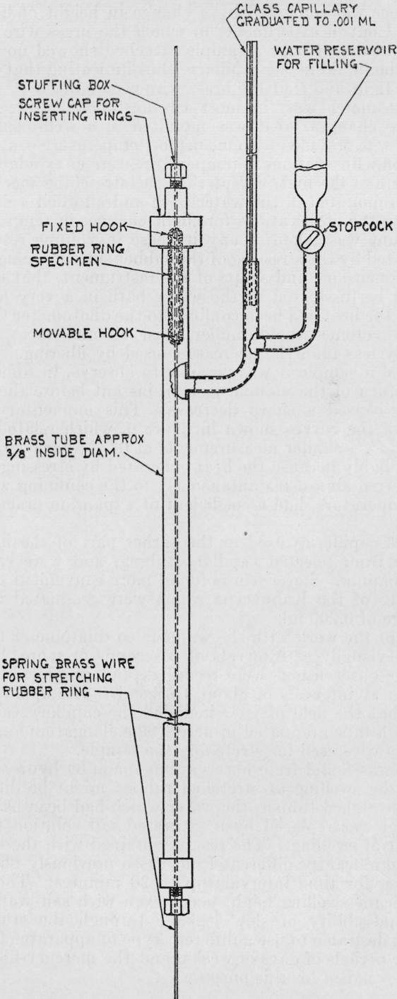
FIGURE 2.—Water-filled dilatometer for measuring the change of volume of rubber on stretching.
