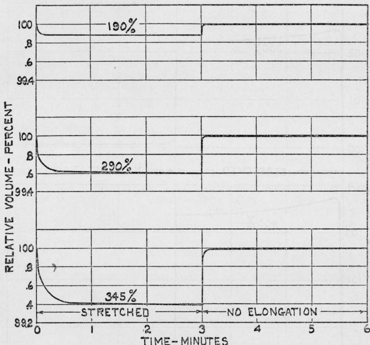
FIGURE 5.—Changes in volume of compound IV (containing 10 percent, by volume, of carbon black) when stretched and when released.
