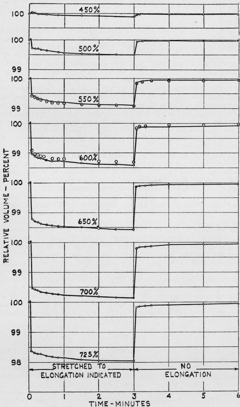
FIGURE 6.—Change in volume of rubber on stretching to different elongations at 25° C.
