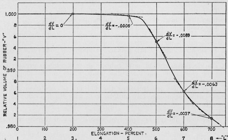
FIGURE 13.—Elongation-volume relation for use in computing Poisson's ratio
