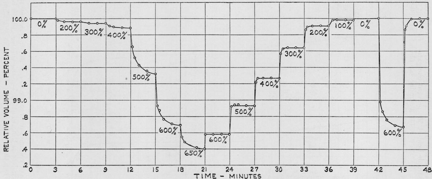
FIGURE 7.—Change in volume of rubber when stretched and when released in a stepwise manner
