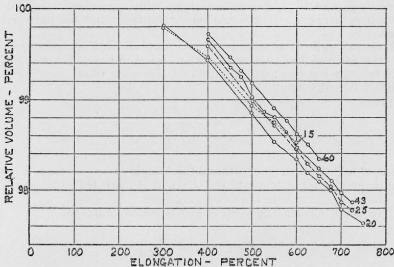
FIGURE 12.—Effect of time of vulcanization on the change in volume of rubber when stretched to different elongations.
