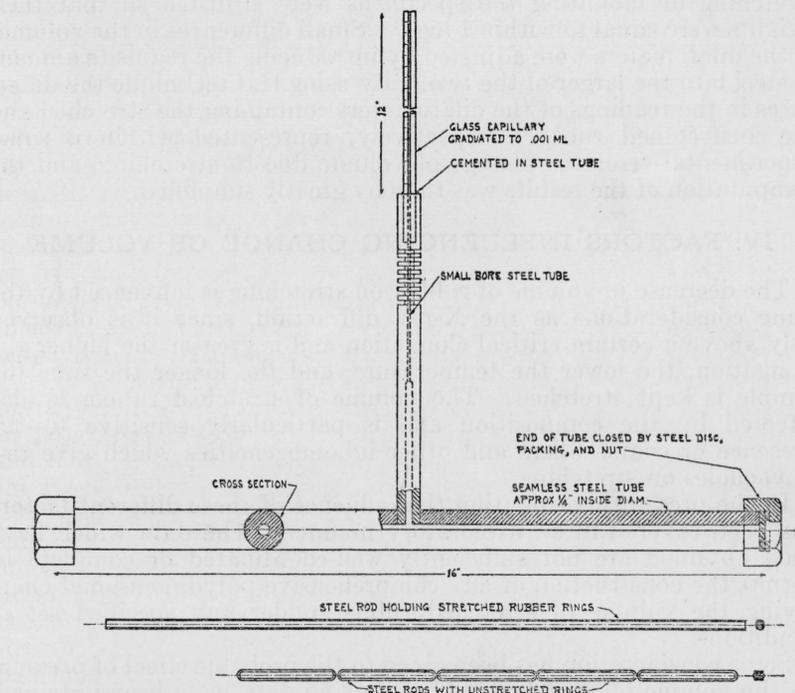
FIGURE 3.—Mercury-filled dilatometer for measuring the change of volume of stretched rubber over long periods of time.
