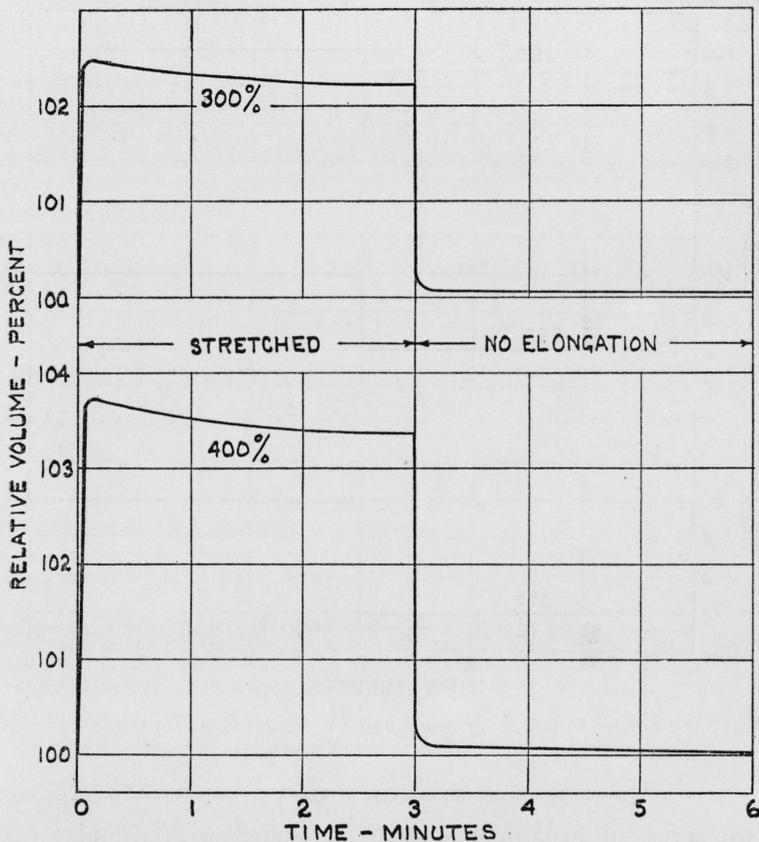
FIGURE 4.—Changes in volume of compound III (containing 10 percent, by volume, of whitening) when stretched and when released.
