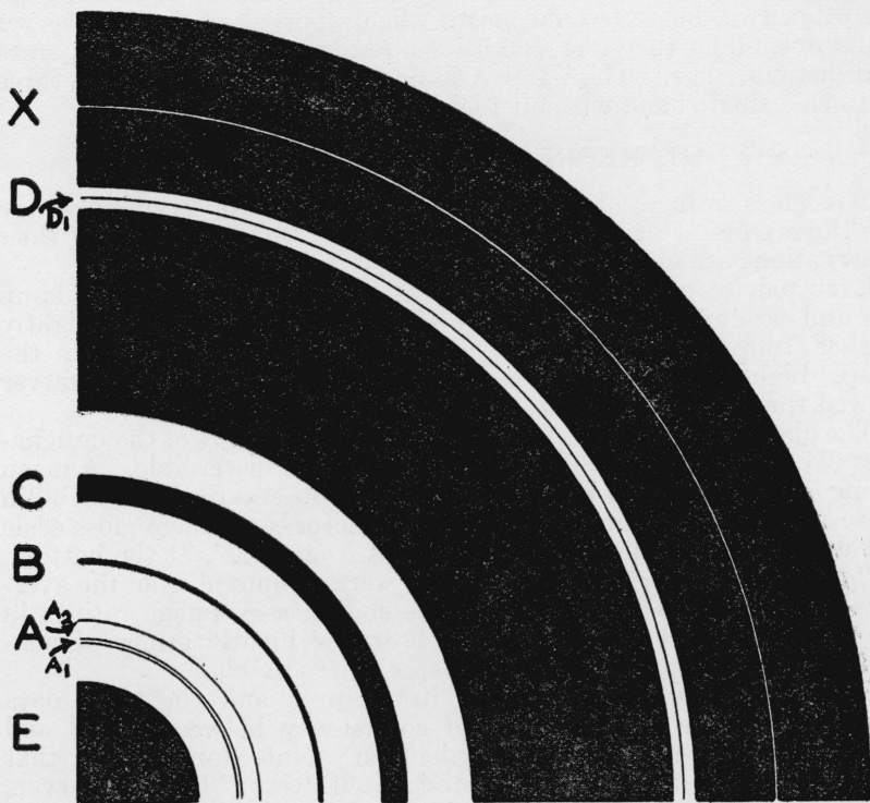
FIGURE 2.—One-quarter circle of the target pattern reproduced full scale, with letters to identify the different rings and lines.
