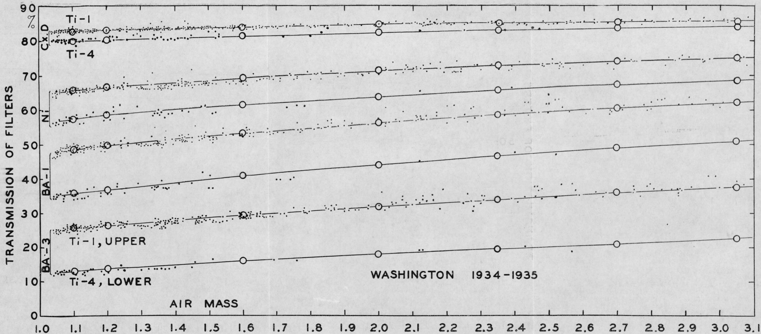
FIGURE 2.—Diurnal variation in transmission of ultraviolet solar radiation through standard filters (see figure 1) observed at Washington. The large circles are the calculated transmissions for ultraviolet spectral-energy curves identified with the corresponding air masses, see figure 9. The black dots represent observed values.
