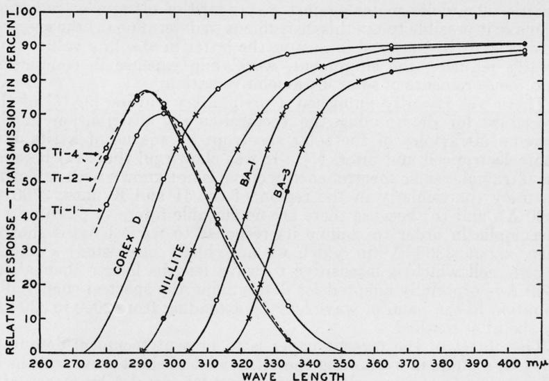
FIGURE 1.—Relative response curves of titanium photoelectric cells Ti-1, Ti-2, and Ti-4 to an equal-energy spectrum; also spectral transmission of glass filters used (Corex D, Nillite; both trade names); and barium-flint glass (Ba-1 and Ba-3; thickness 1 mm and 3 mm, respectively).
