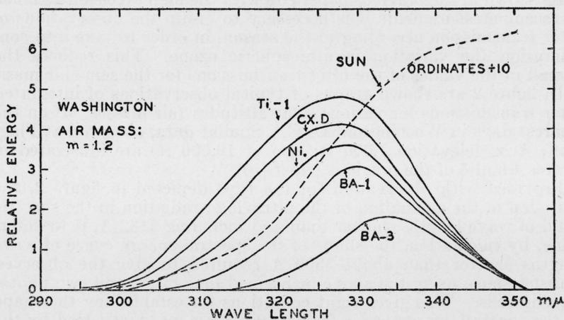
FIGURE 3.—Spectral-energy curve of the sun as it would be observed with a non-selective radiometer and with a selective photoelectric radiometer, Ti-1, without a filter, and through the standard filters Ba-3, etc.
