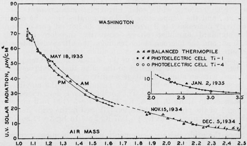
FIGURE 6.—Measurements of ultraviolet solar-radiation intensities at Washington, showing the agreement in the results obtained by two methods of evaluation: (1) by means of a balanced thermopile and filter radiometer, calibrated against a standard of thermal radiation, and (2) by means of a photoelectric ultraviolet meter, calibrated against a standard of ultraviolet radiation.
