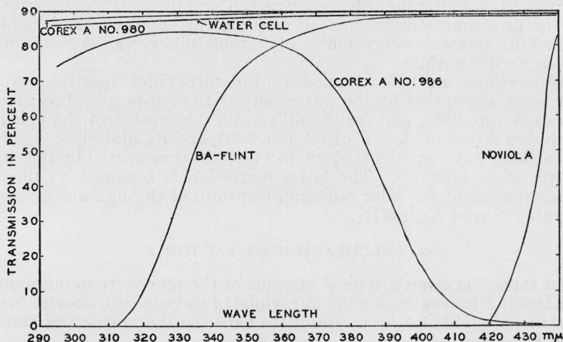
FIGURE 4.—Transmission of filters used in the balanced-thermopile and exclusion-filter method of evaluation of ultraviolet.
