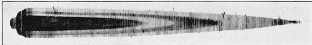
FIGURE 6.— Cut produced on composite coating of nickel, copper, nickel on steel ( \times 2 ). Total thickness 0.002 inch. The dark center portion is the exposed steel that has been treated with copper sulphate to produce contrast. The next dark area is the copper layer between two nickel layers.
