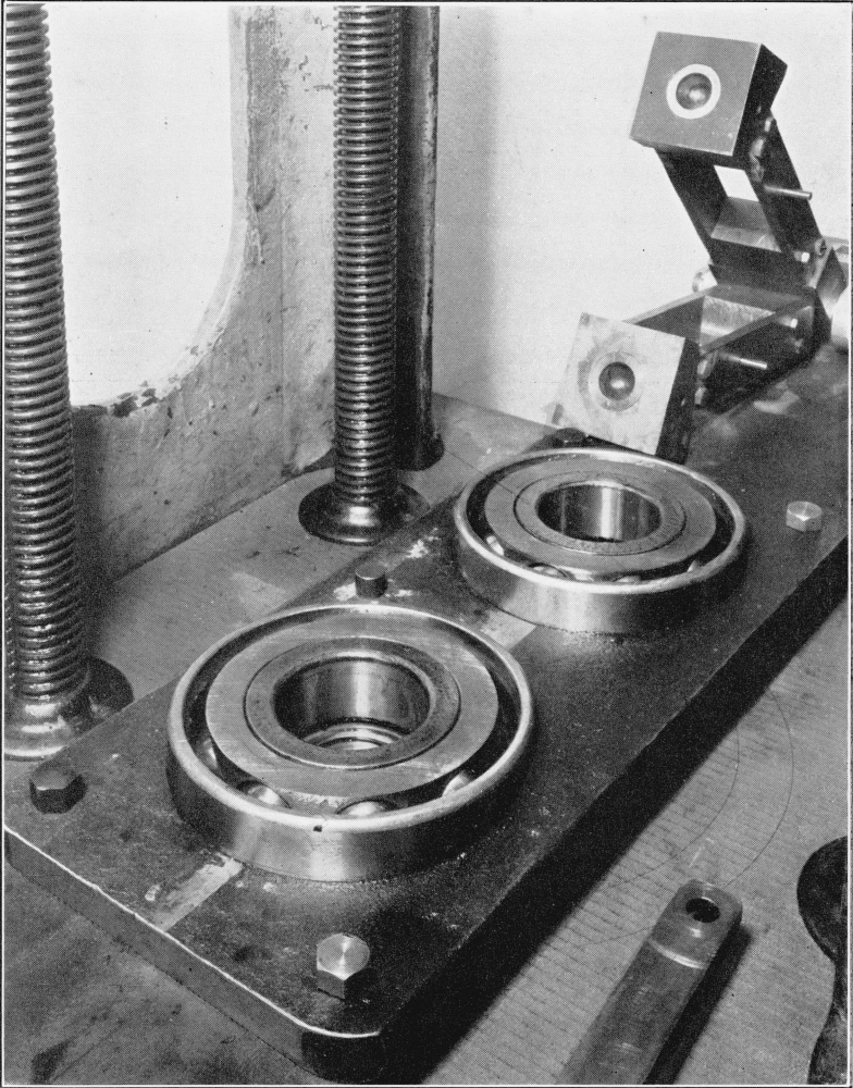
FIGURE 4.— Combination thrust and radial bearings and the cup-holding assembly.
